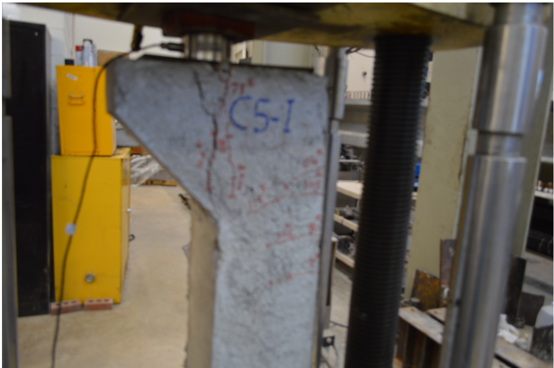
Figure B8 Specimen C5-I under applied load
