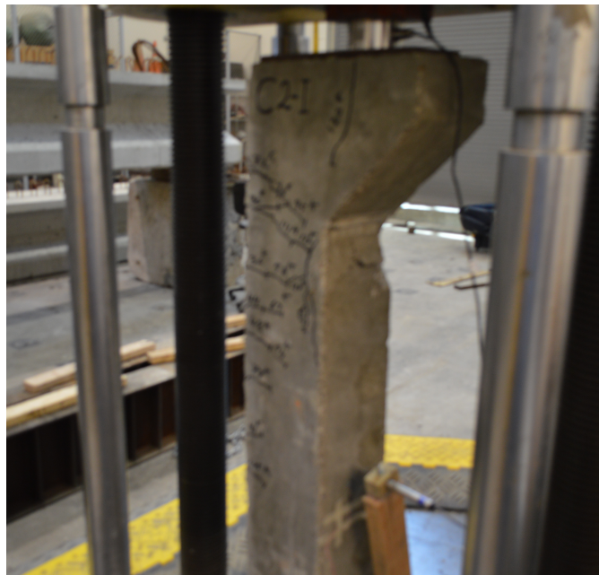
Figure B10 Specimen C2-I under applied load
