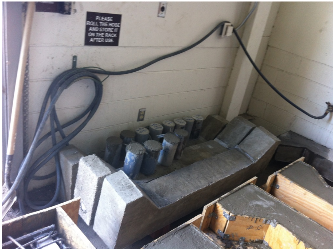
Figure B6 Concrete Specimen being casted at the Laboratory
