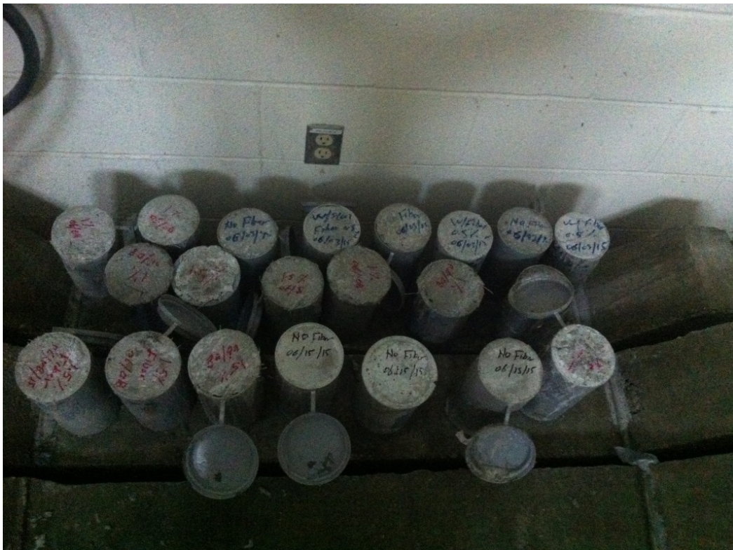
Figure B5 Concrete Cylinders for various specimens
