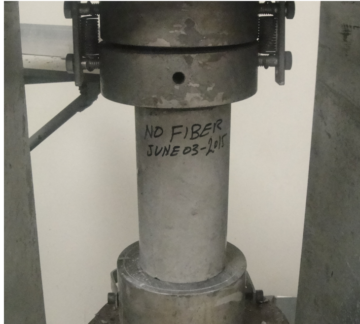
Figure B1 Concrete Cylinder of specimens containing 0% steel fibers
