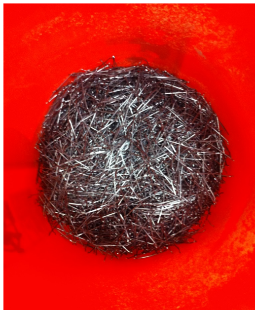
Figure 3.4 Steel Fibers used in the experiment (Azzawi 2017)
