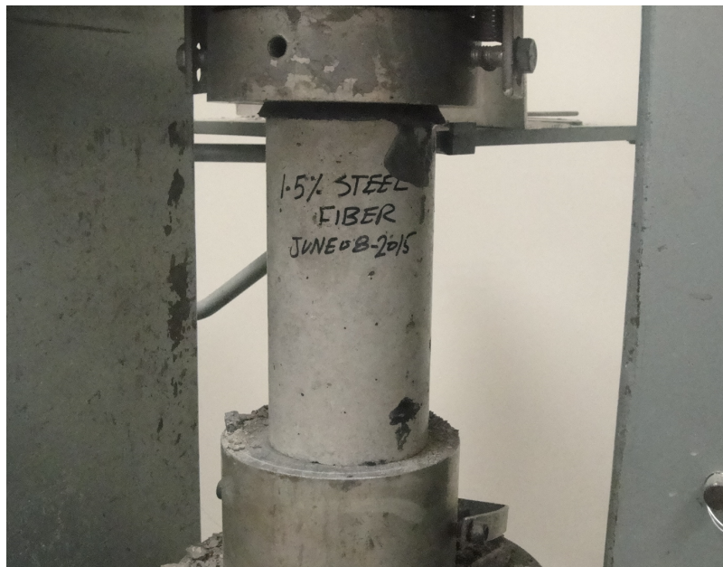
Figure B4 Concrete Cylinder of specimens containing 1.5% steel fibers
