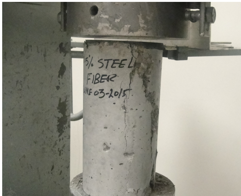
Figure B2 Concrete Cylinder of specimens containing 0.5% steel fibers
