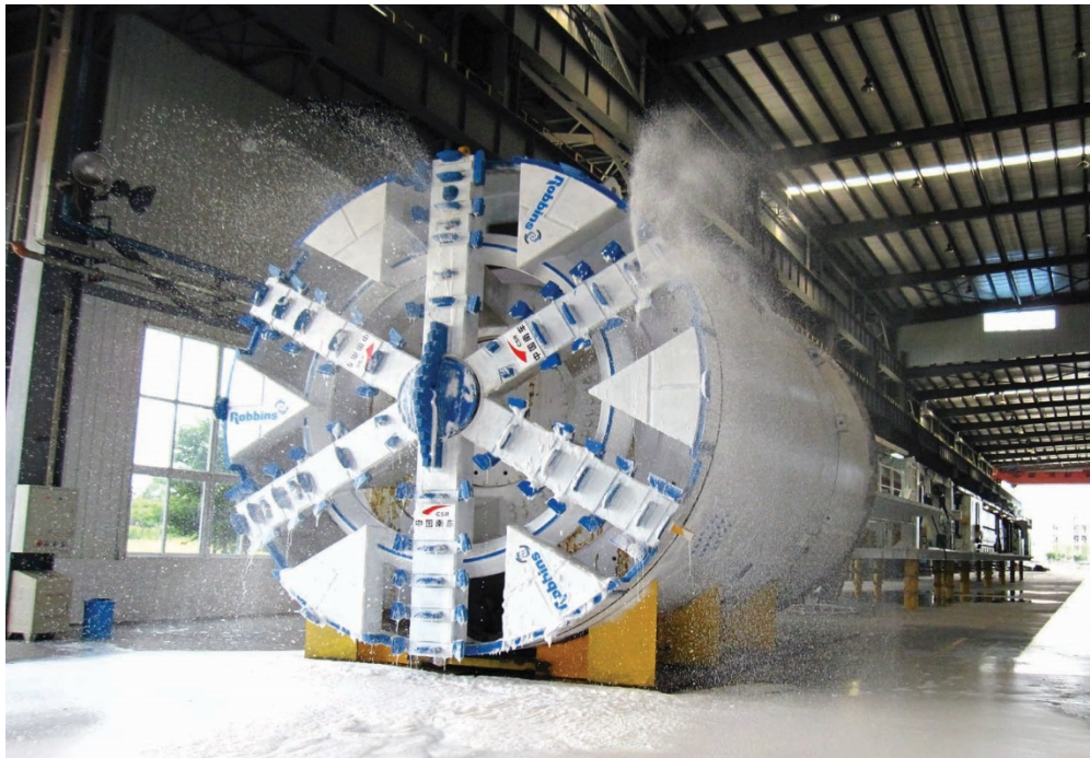
Figure 5-13 Robbins 20.6 ft Diameter EPB Used for Zhengzhou Metro Line 1
