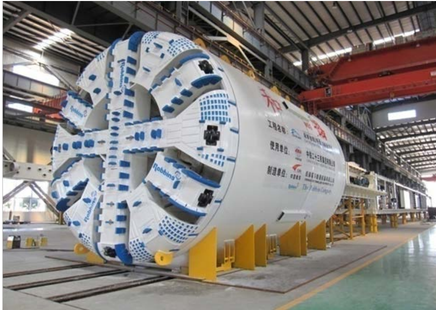
Figure 5-8 Robbins 20.53 ft Diameter EPB Used on Line 2
