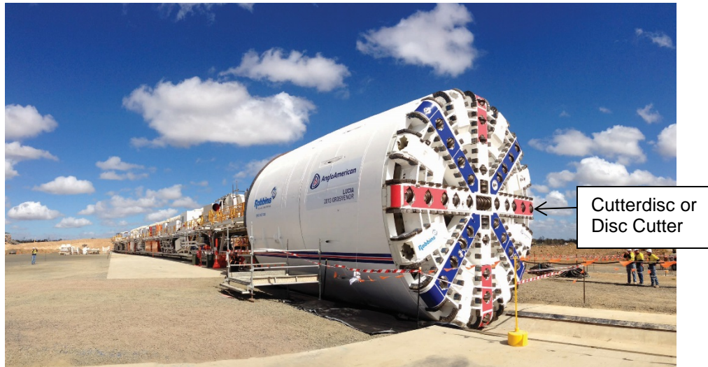
Figure 2-12 EPB TBM with Cutterdiscs and Drag Picks (Robbins, 2017b)
