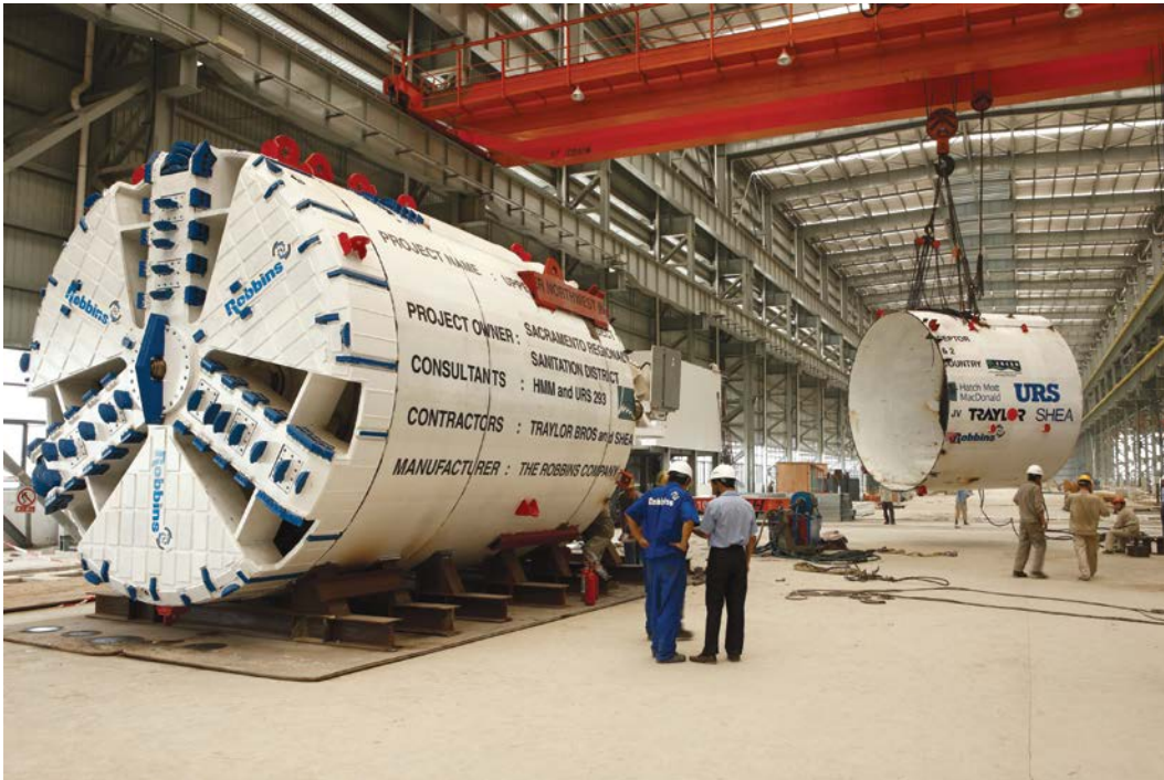
Figure 5-12 Robbins 13.9 ft Diameter EPB in the Shop
