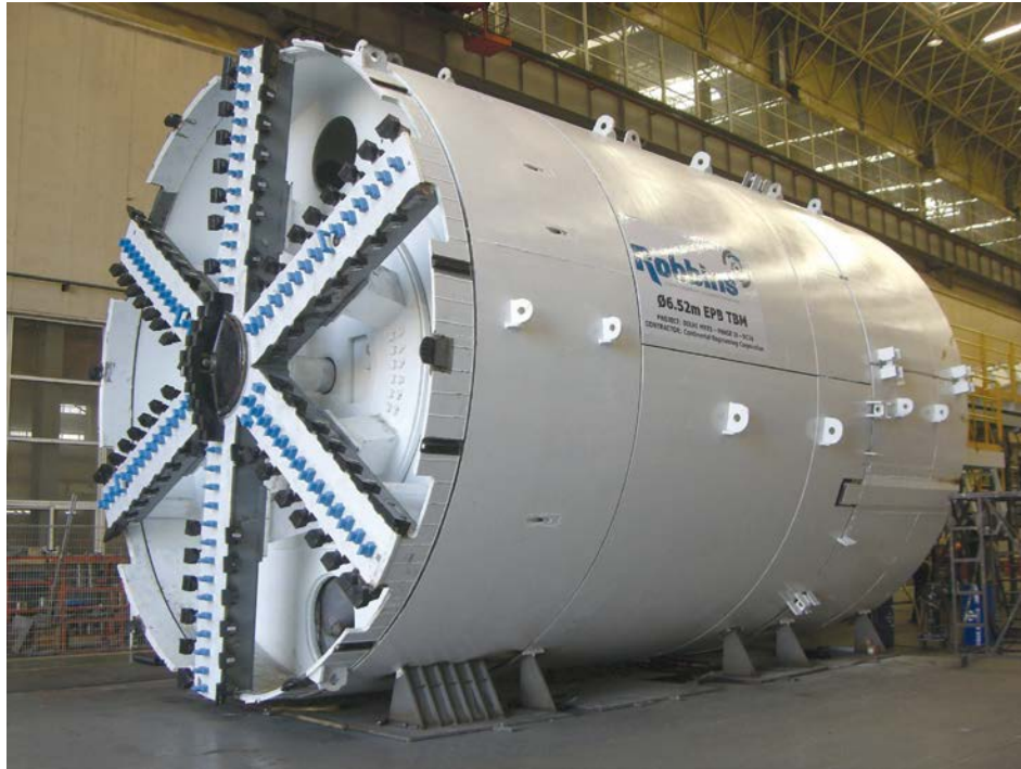
Figure 5-11 Robbins 21.4 ft Diameter EPB in the Shop
