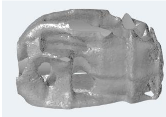
Figure 12: Optimized result imported as an STL file
