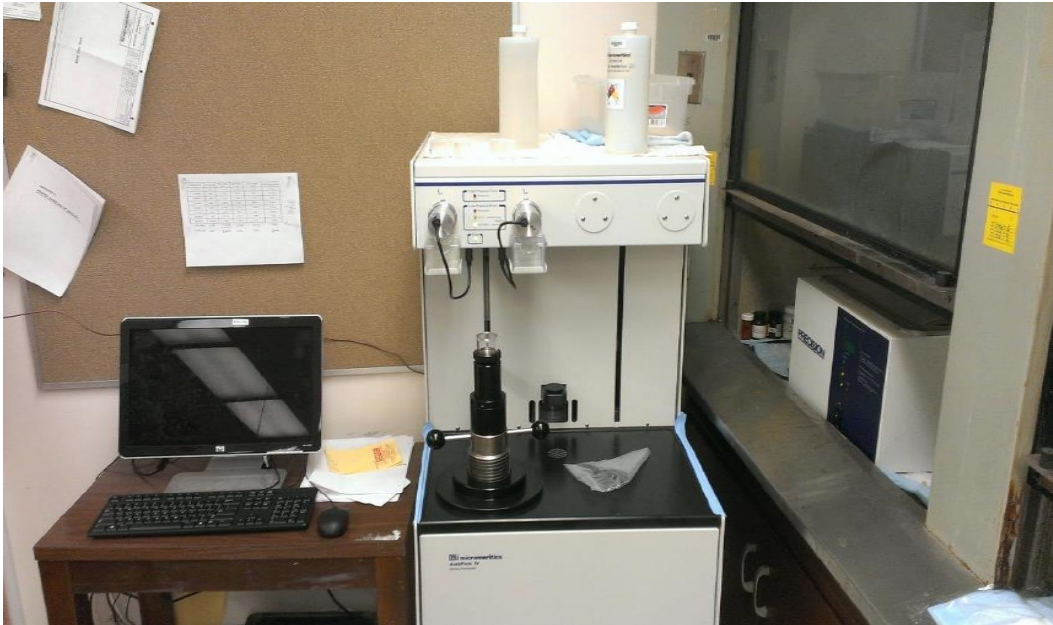
Figure 4-25. AutoPore IV 9510 used for the Mercury Intrusion Analysis; Image taken from Zastoupil (2015)
