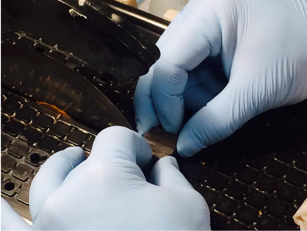
Figure 4-23. Sample preparation for Mercury Intrusion Porosimetry. Samples were cut in 3x3x3 cubes for testing
