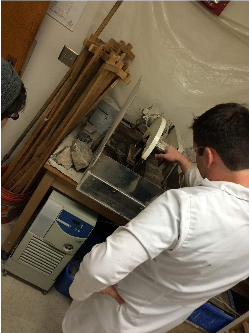
Figure 4-19. Preparing samples for acoustic testing using the Water Saw in the UTA
