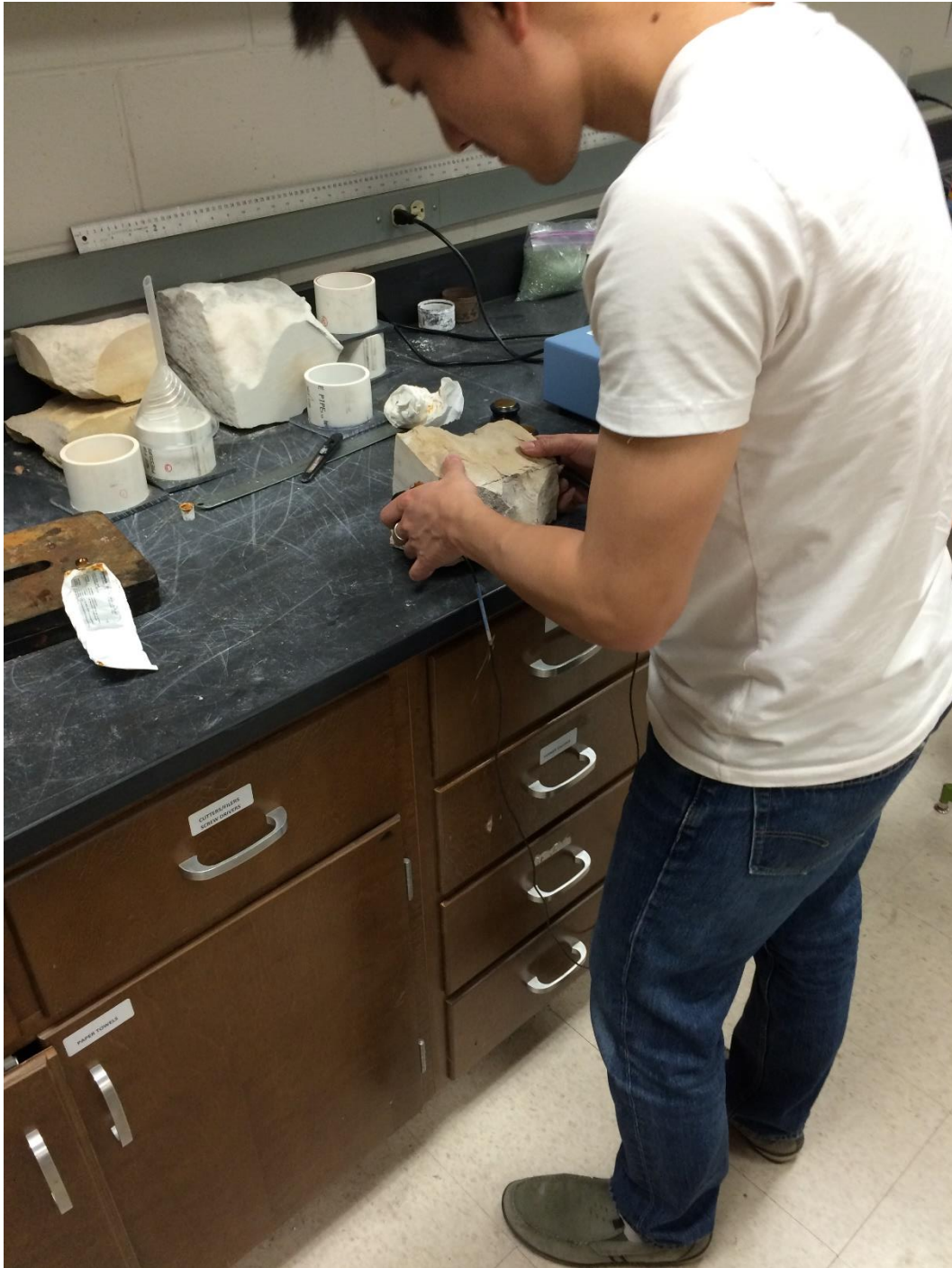
Figure 4-22. Measuring acoustic wave velocities using the ATSM 2845
