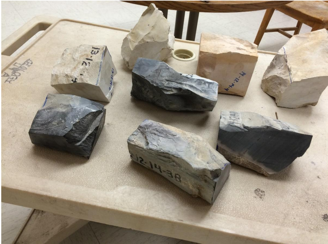
Figure 4-20. Example of samples cut with smooth, parallel surfaces perpendicular to bedding in order to optimize acoustic velocity measurements
