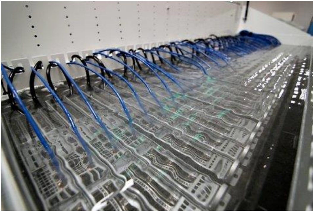
Figure 1.3 Oil Immersion cooling
