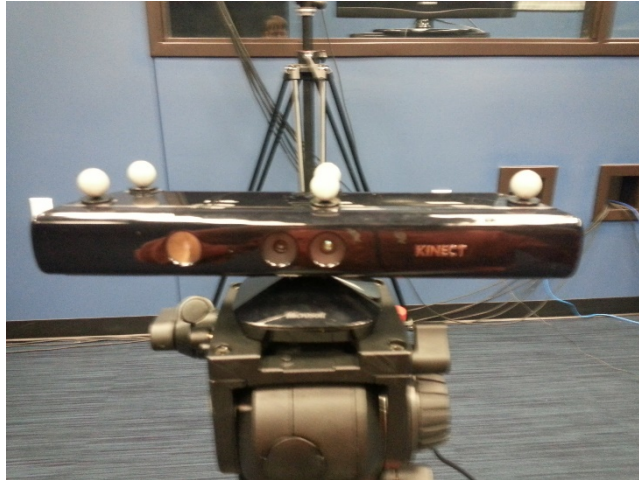
Figure 3.2 The Microsoft Kinect Sensor with Vicon markers placed on top
