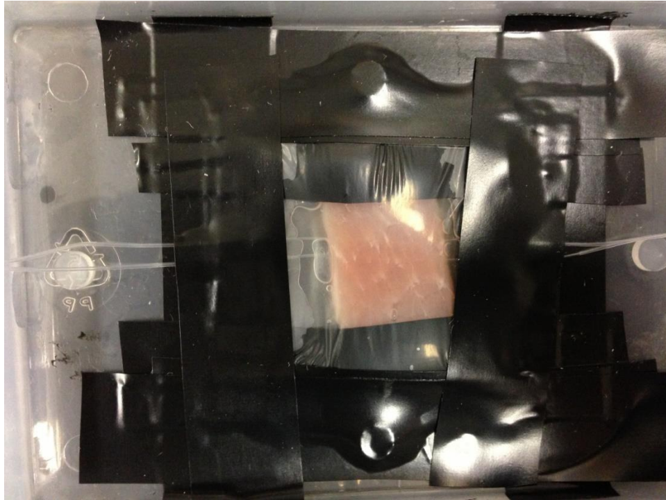
Figure 5-2 The tissue phantom setup for two-color USF imaging.
