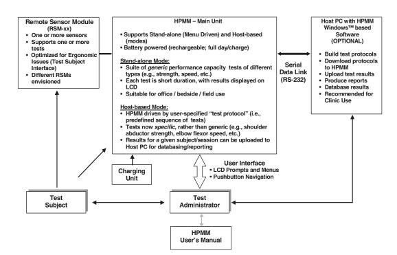
Figure 2.1 Major Features of the Overall HPMM System Concept.
