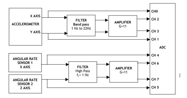
Figure 3.3 Conceptual Block diagram for Acceleration and Angular Rate Subsystems.
