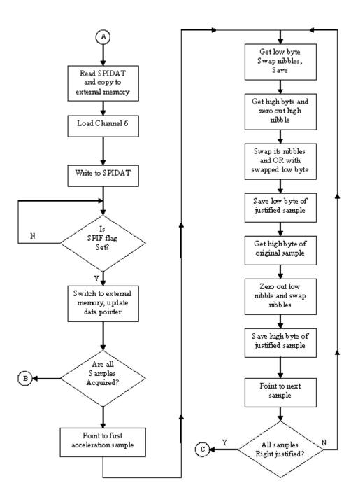
Figure 3.10 Flowchart (part 2) for GTA 6: Hand-Arm Steadiness Test.
