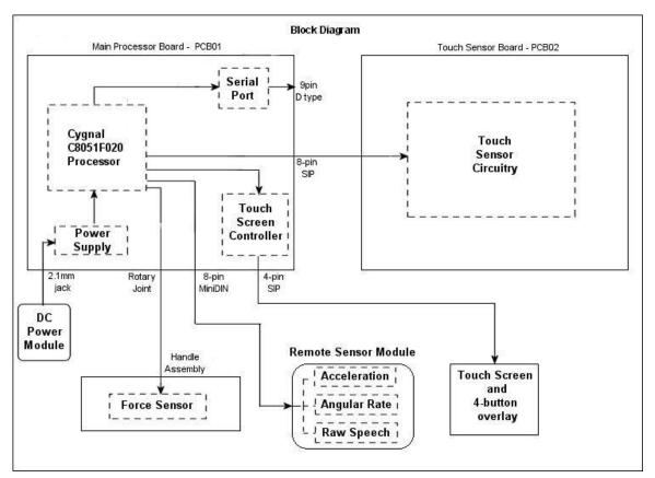
Figure 2.2 HPMM System Block Diagram.
