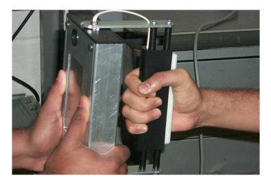
Figure 4.2 HPMM Position for the Grip Strength Test.
