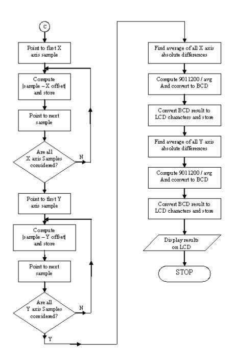
Figure 3.11 Flowchart (part 3) for GTA 6: Hand-Arm Steadiness Test.
