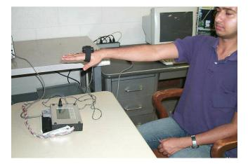
Figure 4.7 Hand-Arm Posture for Steadiness Test.
