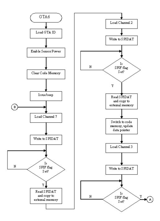
Figure 3.9 Flowchart (part 1) for GTA 6: Hand-Arm Steadiness Test.
