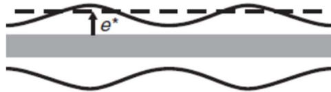
Figure 3: Cross-sectional view of a liquid film coated on a fiber
