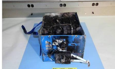
An auxiliary power-unit battery from a Boeing 787 caught fire at Logan Airport... (National Transportation...)
