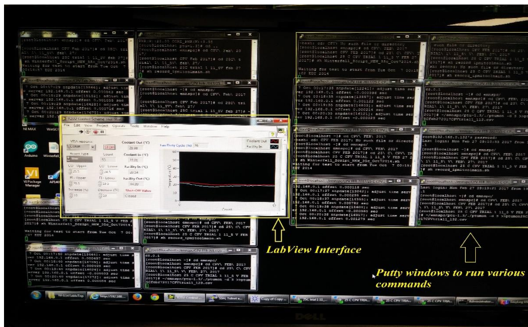
Figure 5-2 Commands in Putty Software for Data Collection using IPMI and PTU tools
