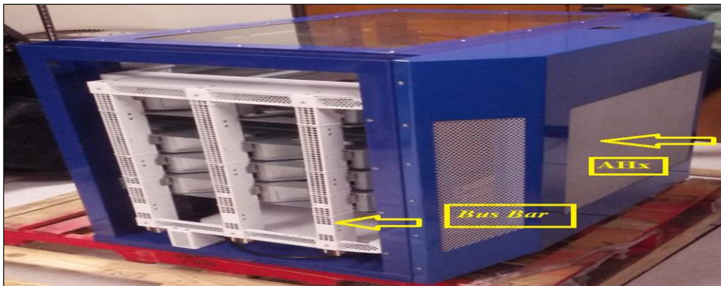
Figure 2-12 AHx Unit by CoolIT Systems [17]
