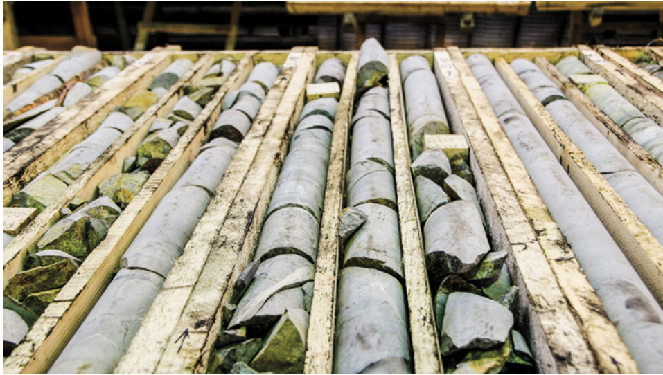
Figure 2-6 Rock Core Samples in Core Box (ALS Global 2017)
