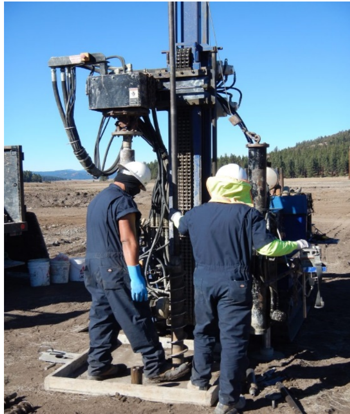
Figure 2-4 Vertical Test Boring/Rock Coring (Devin, 2016)
