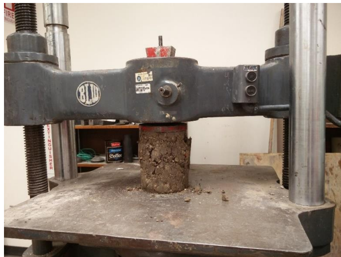
Figure 3-8 Sample specimen at failure
