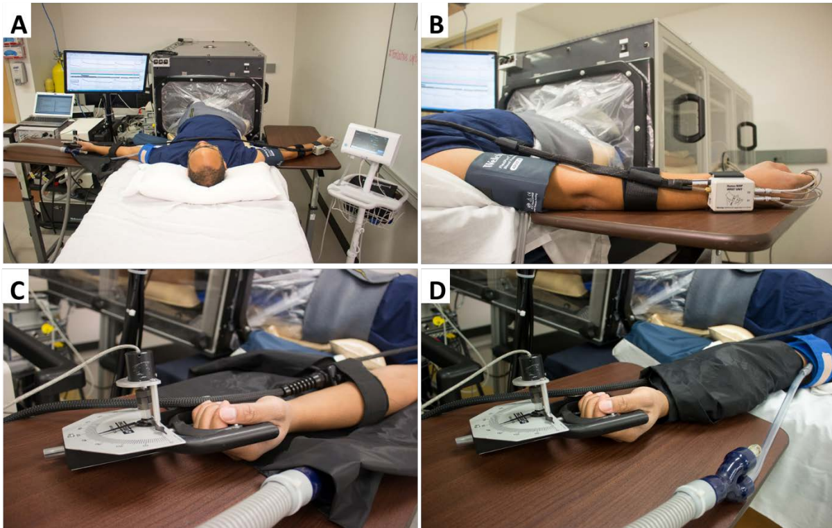
Figure 1. Experimental set-up and instrumentation. (A) Representative experimental set-up, with a typical subject lying supine on a bed with their legs inside the LBNP chamber and fully instrumented. (B) Dominant arm instrumented with a non-invasive beat-to-beat blood pressure device for beat-to-beat arterial blood pressure measurement, and a brachial artery blood pressure cuff for calibration and verification of the beat-to-beat system. (C) Instrumentation of the non-dominant arm. The hand is comfortably gripping a handgrip dynamometer (connected to data acquisition system), and the forearm muscle is instrumented with the near-infrared spectroscopy probe. (D) Once instrumented, the NIRS optodes are covered with a black vinyl cloth (to eliminate interference from ambient light). In addition, a rapid cuff inflation system is placed over the brachial artery.
