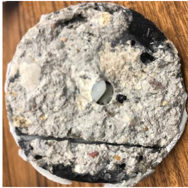
Figure 80 Beam 11, ASTM Pull off test Mode F
