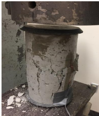
Figure 82 Laboratory test to determine the crushing strength
