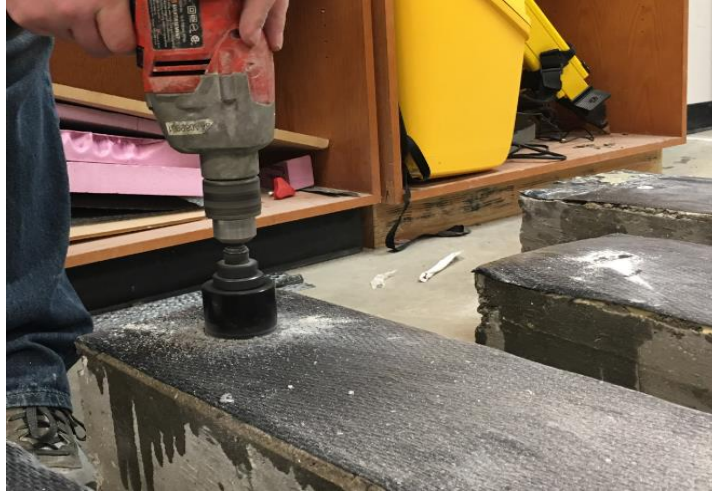
Figure 74 Scoring through the coating
