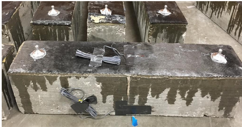
Figure 75 Fixtures attached to the beam samples for pull off test
