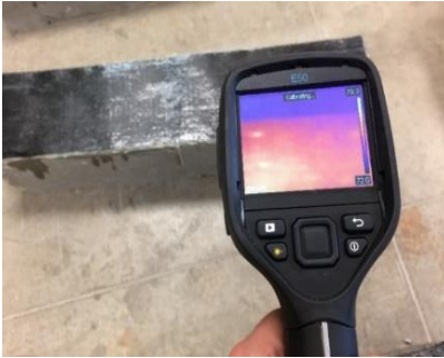
Figure 40 Capturing image after heating the beam
