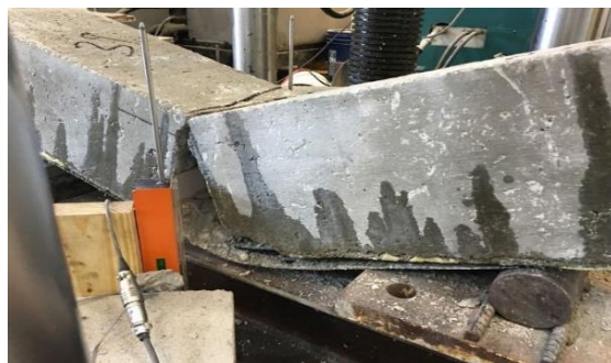
Figure 86 Intermediate crack induced interfacial debonding
