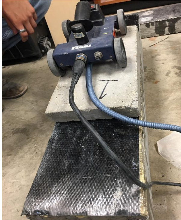
Figure 23 GPR Scan over a sample beam using a concrete additional layer
