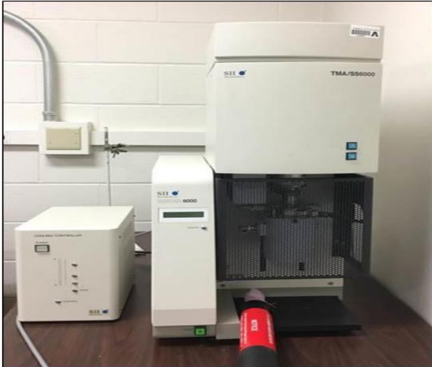
Figure 3.1 Thermal Mechanical Analyzer to measure CTE
