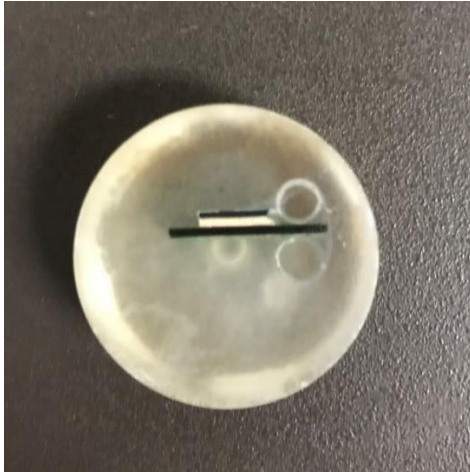
Figure 6.12 Package sample in epoxy mold after polishing.
