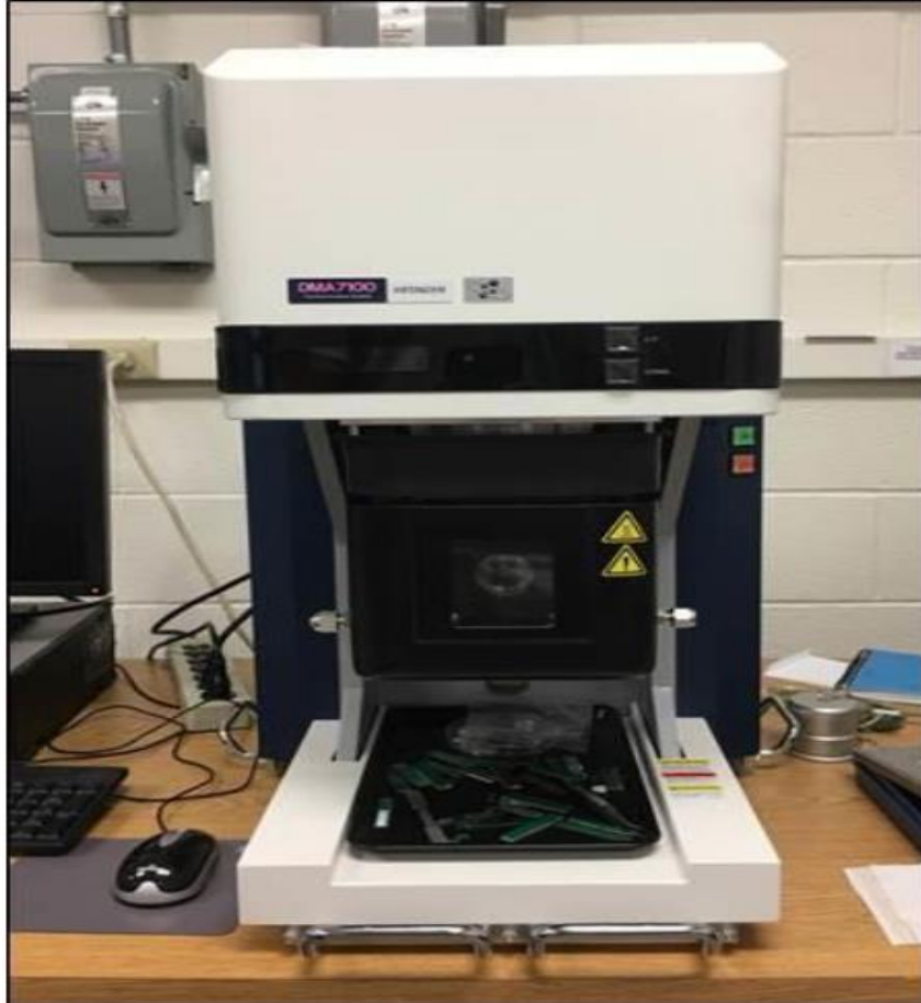
Figure 3.2 Dynamic Mechanical Analyzer to measure Youngs Modulus
