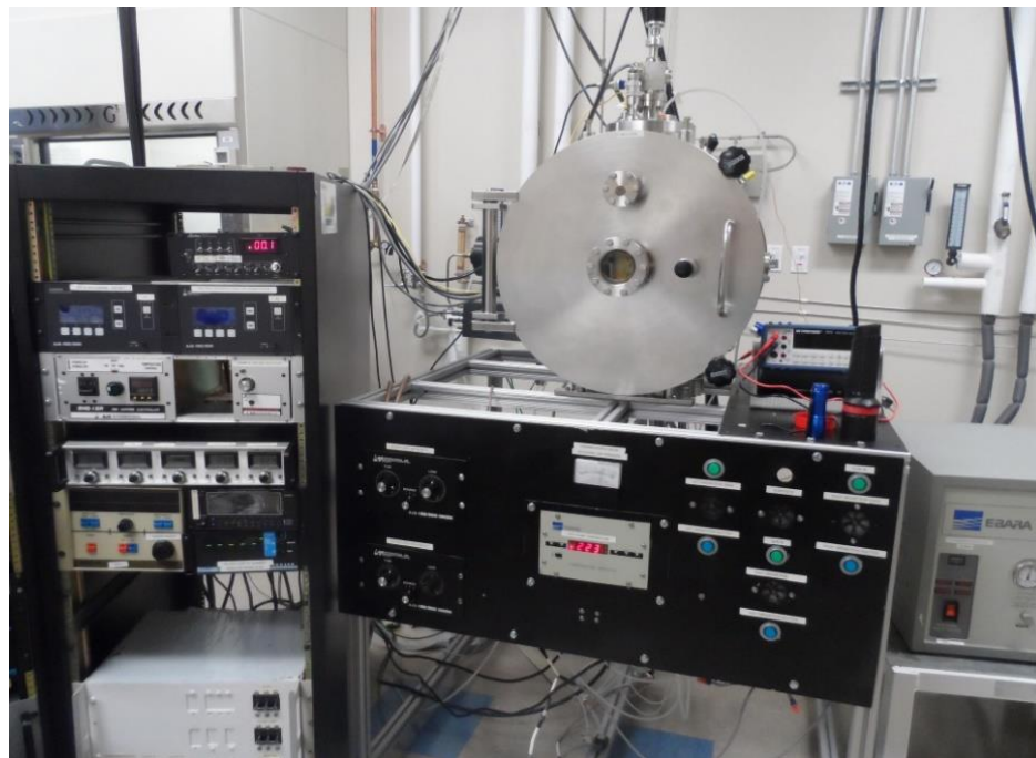
Figure 3-1 PVD reactive magnetron sputtering system in Surface and Nano Engineering Laboratory.
