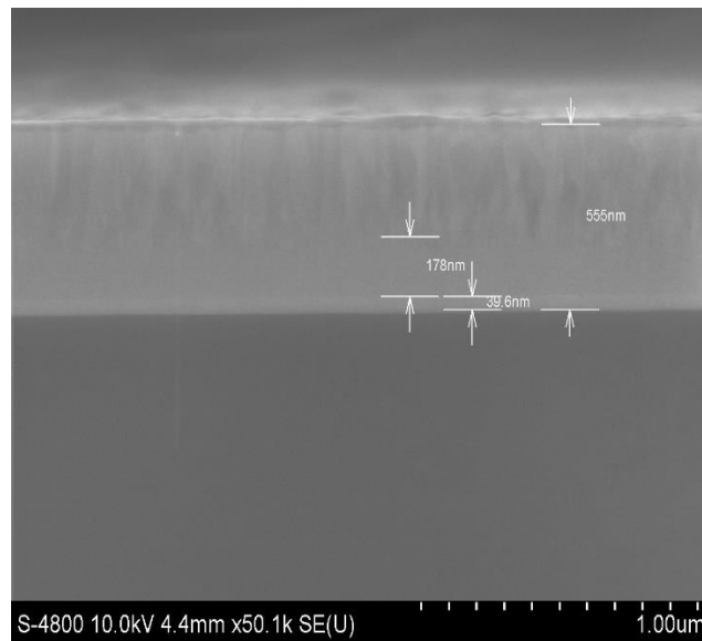
Figure 4-12 Cross section of the Ta–N film deposited with 3% N 2 .
