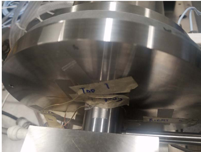
Figure 5-16 Thermocouples Installation at the Back late
