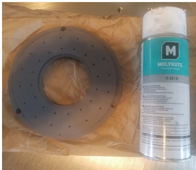
Figure 5-10 Molybdenum Disulfide Coating on the Thrust Air Foil Bearing
