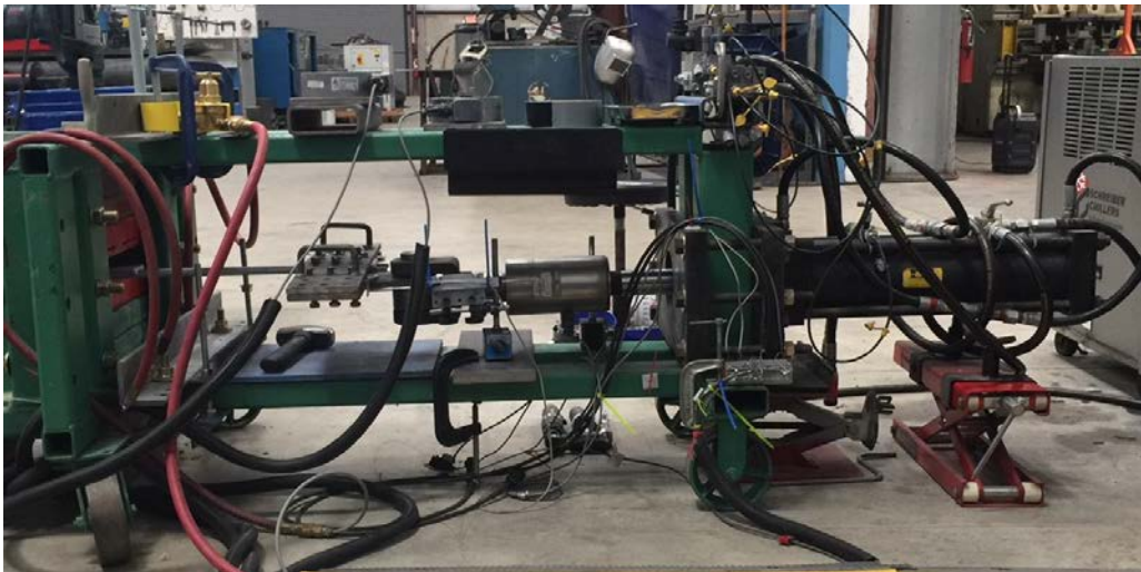
Photograph 3-5 Horizontal Load Frame
