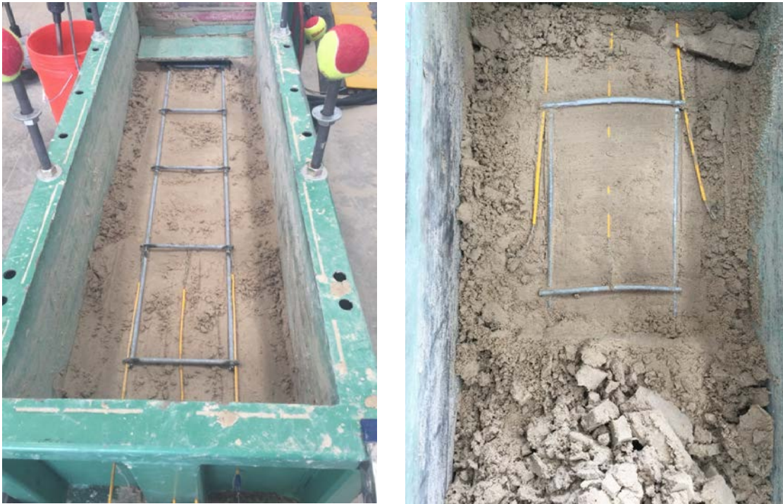
Photograph 4-3 Transverse Bar Bending in MW71 x MW71 – 200 x 300
