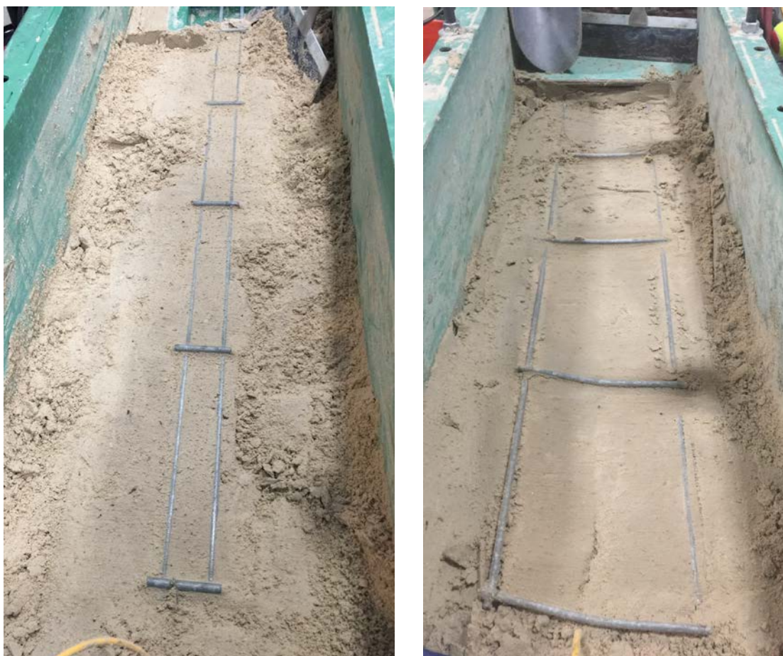
Photograph 3-28 Exhuming Soil-Reinforcing Element After Test
