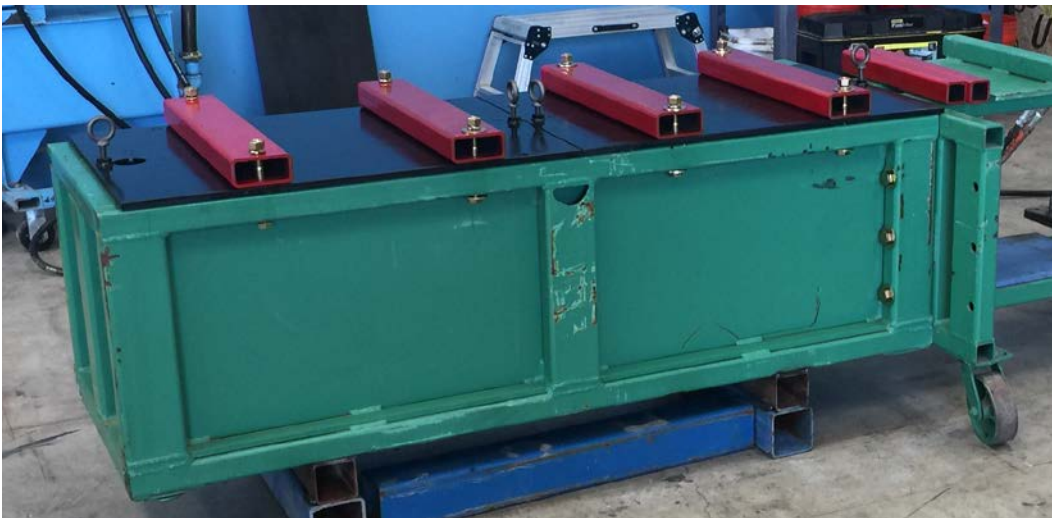
Photograph 3-2 Pullout Box with Closed-Mount
