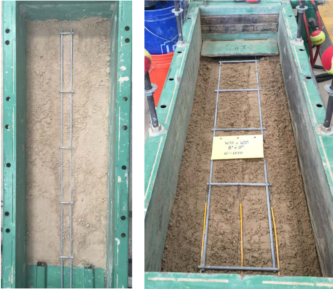
Photograph 3-18 Placement of Soil-Reinforcing in Soil-Box
