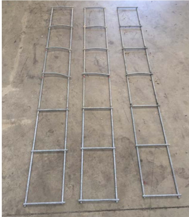
Photograph 3-29 Exhumed Soil-Reinforcing Element After Test
