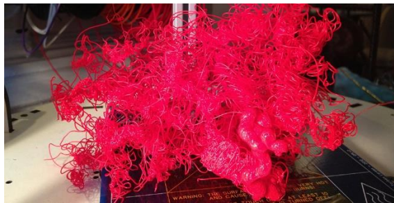
Figure 7: Defects (Spaghetti patterns) due to improper bonding [29]
