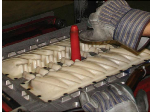
Figure 4 Sand casting through additive manufacturing [9]
