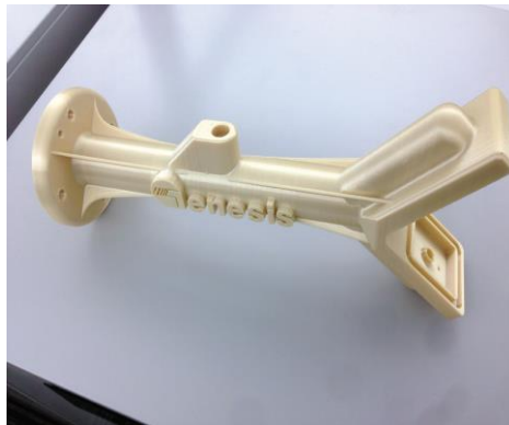
Figure 3: A lightweight FDM end effector by Genesis Systems Group [9]
