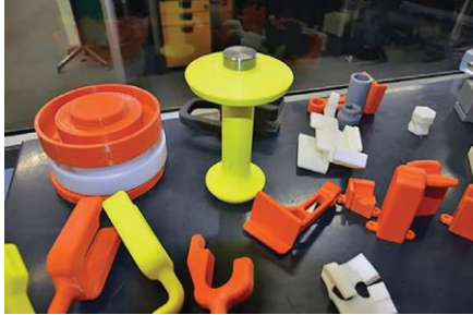
Figure 2: Jigs and Fixtures additively manufactured by Volvo [8]
