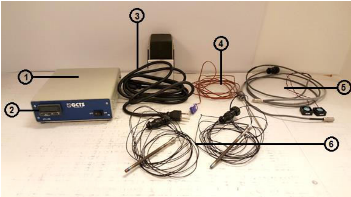
Figure 3-6: GCTS HTC 250 Heat controller and components. 1) GCTS HTC-250 heat controller, 2) Omega CN132 temperature controller, 3) power cable, 4) Omega Type E thermocouple, 5) 2 Orion 12V DC fans, and 6) 2 120V heating elements.
