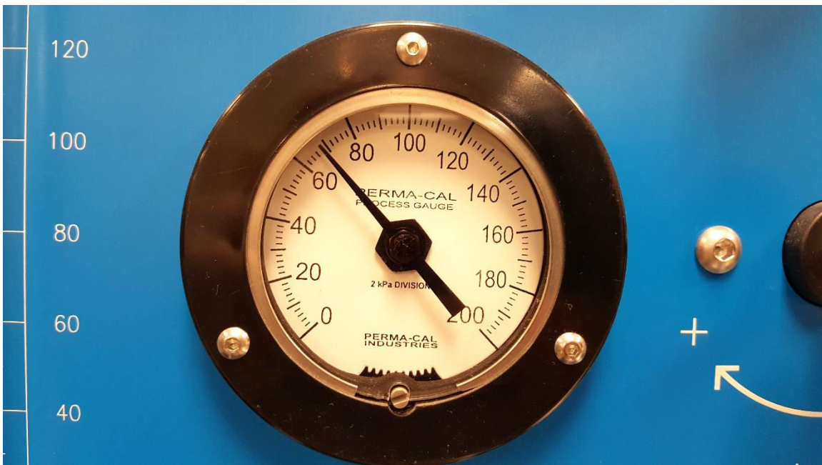
Figure 5-4: Resonant column confinement pressure gauge set to 68 kPa.
