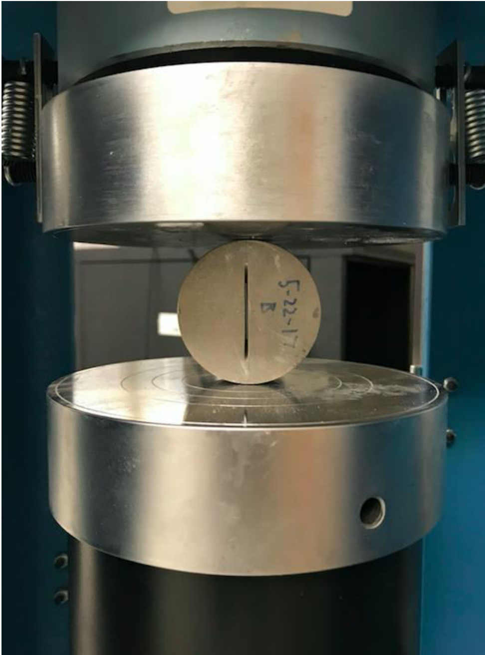
Figure 27 - Example of final specimen geometry and how testing is done in Forney F-325 Compression Testing Machine.
