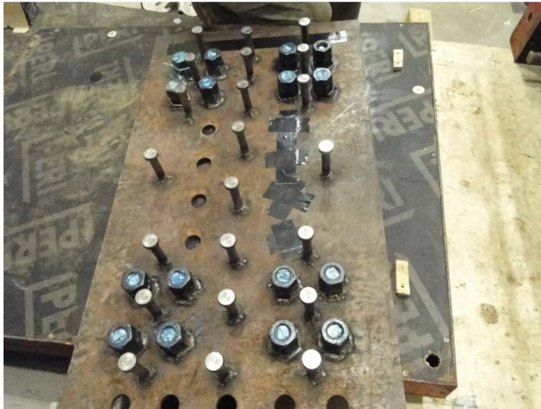
Figure 2.14 Plat with shear studs
