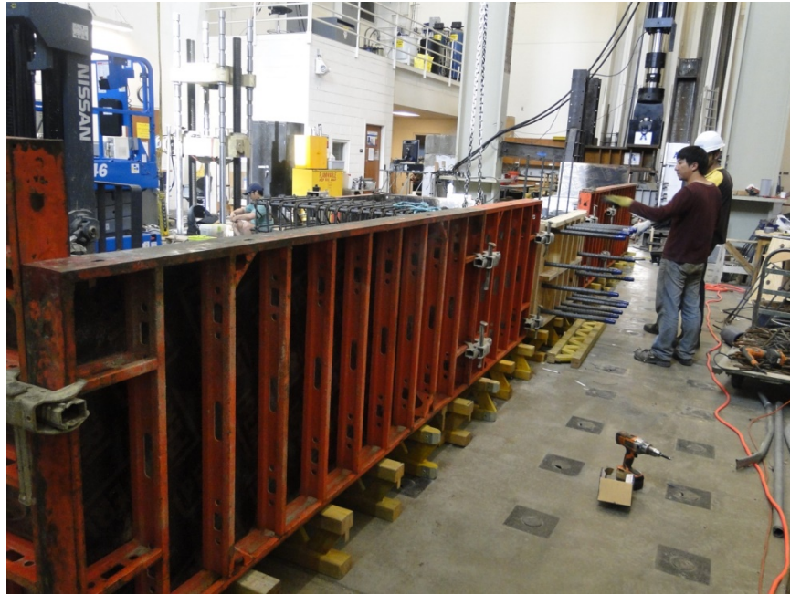
2.19 Formworks for lower part of specimen
