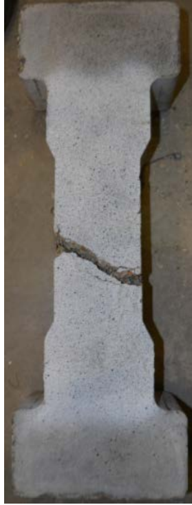
Figure 2.3 HPFRC dog-bone specimen after test
