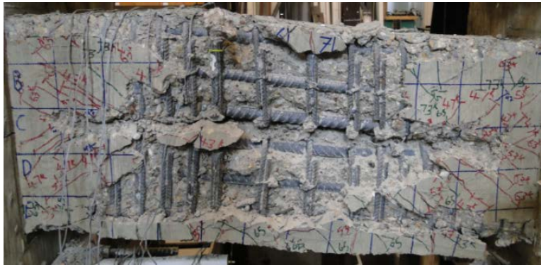
Figure 8.8 (a) Hysteresis response of specimen with 0.25 in.-wide gap and (b) damage pattern at 6% beam chord rotation
