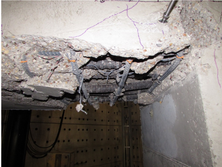
Figure 3.32 Buckled longitudinal reinforcement for RC-SP-CL
