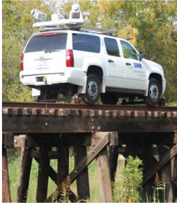
Figure 2-15. Mobile LiDAR to Survey a Railway Line for Asset Inventory (Leslar et al. 2009)
