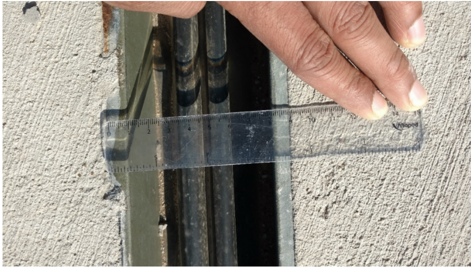
Figure 4-43. Ground Truth Measurement of Joint Width
