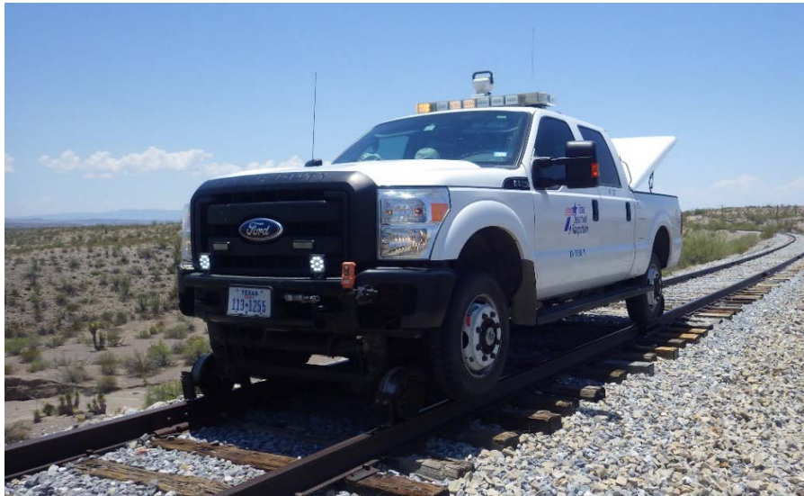
Figure 4-48. Ford F250 Crew Cab Truck Equipped with Hi-Rail Gear
