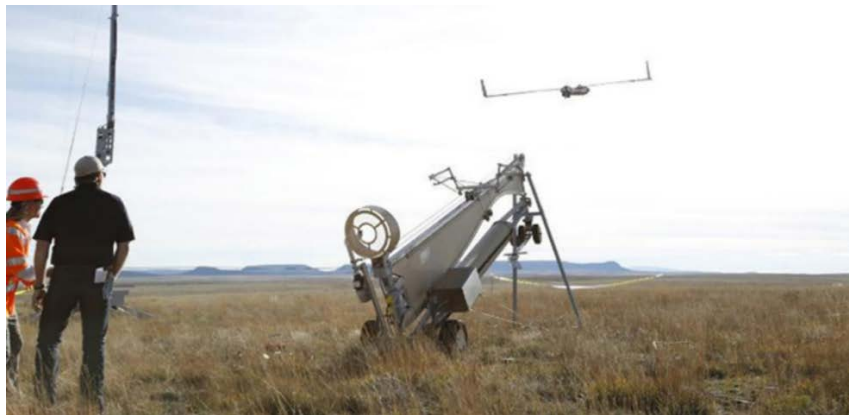
Figure 2-29. BNSF and Insitu Inc. Launching the ScanEagle UAV for Rail Inspection (Insitu 2015)
