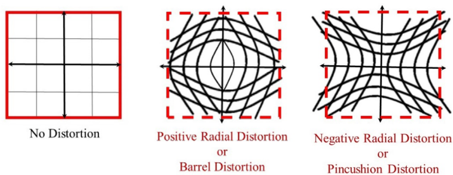
Figure 3-4. Different Radial Distortion Scenarios
