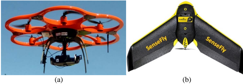
Figure 1-2. Types of UAVs (a) Aibot X6 Multi-rotor (b) SenseFly Ebee Fixed
