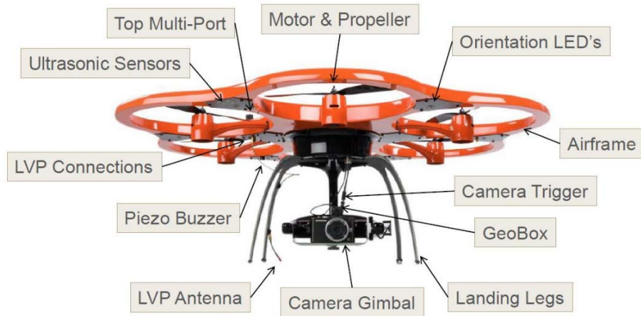
Figure 3-2. Components of Aibot X6 V2 Hexacopter (Source: Leica Geosystems)
