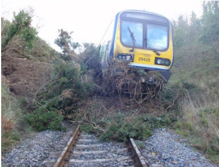
Figure 2-14. Train Derailment Due to Debris on Track (RAIU 2010)
