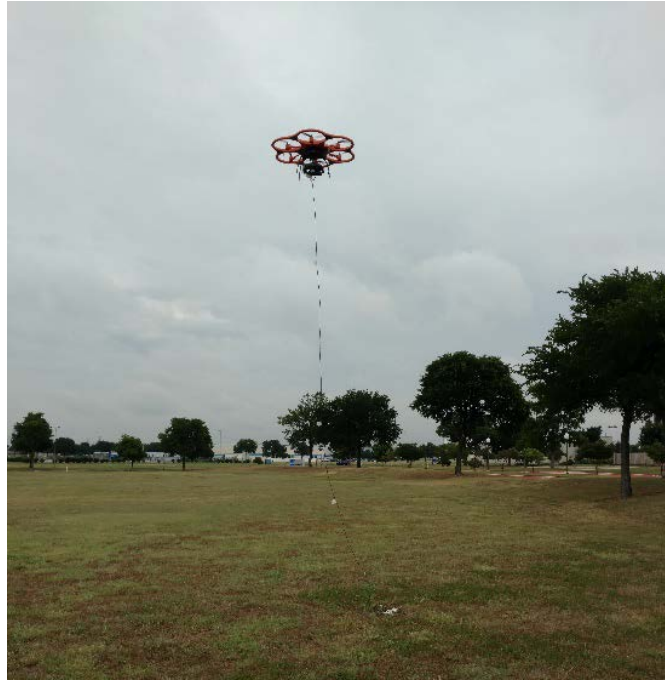
Figure 3-9. Flying UAV Attached with a Lightweight Rope Marked with 1-meter Intervals
