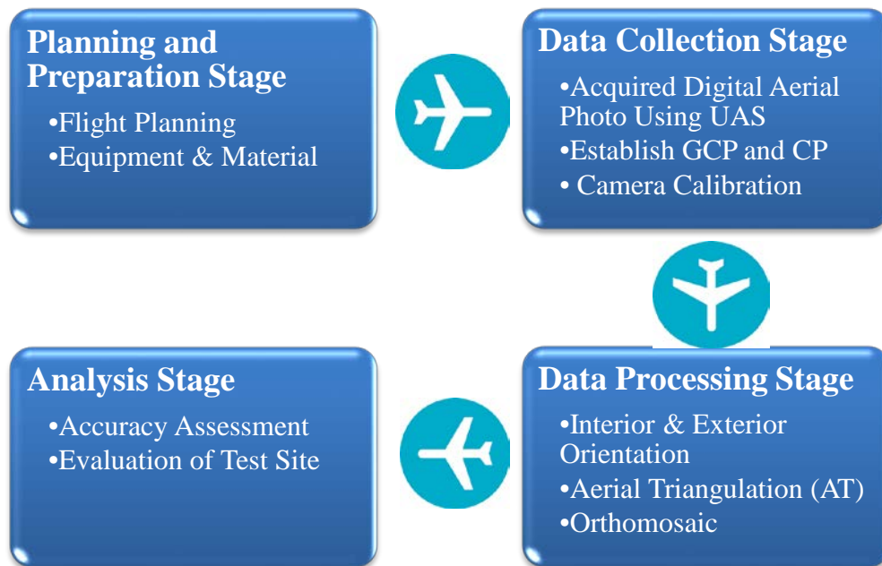
Figure 1-1. Different Stages of the Aerial Photogrammetry Process
