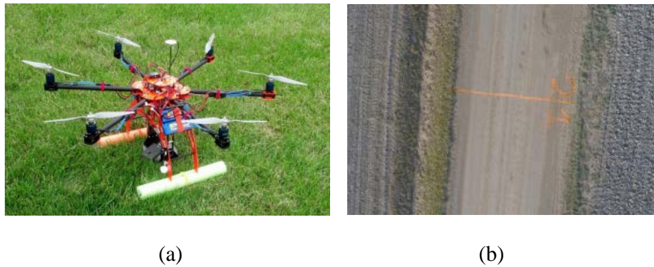
Figure 2-24. Aerial Data Collection (a) UAV with a Digital Camera; (b) High-Resolution Image from UAV Camera (Brooks et al. 2015)
