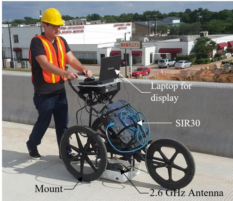
Figure 4-1 Tri-wheel Cart with Ground Coupled Antenna
