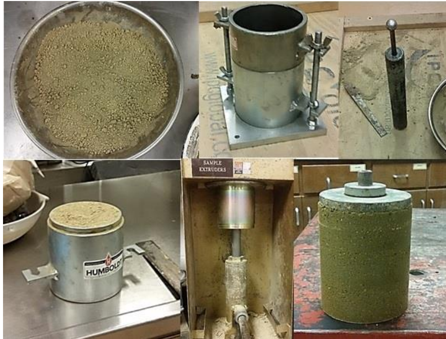
Figure 3-6 Standard Compaction Test
