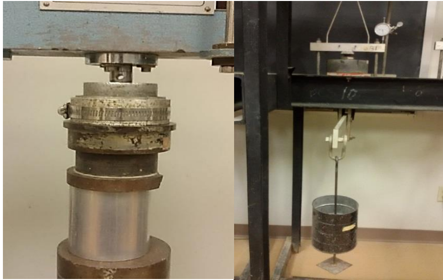
Figure 3-7 Static Compaction of Soil and One-d Swell Test
