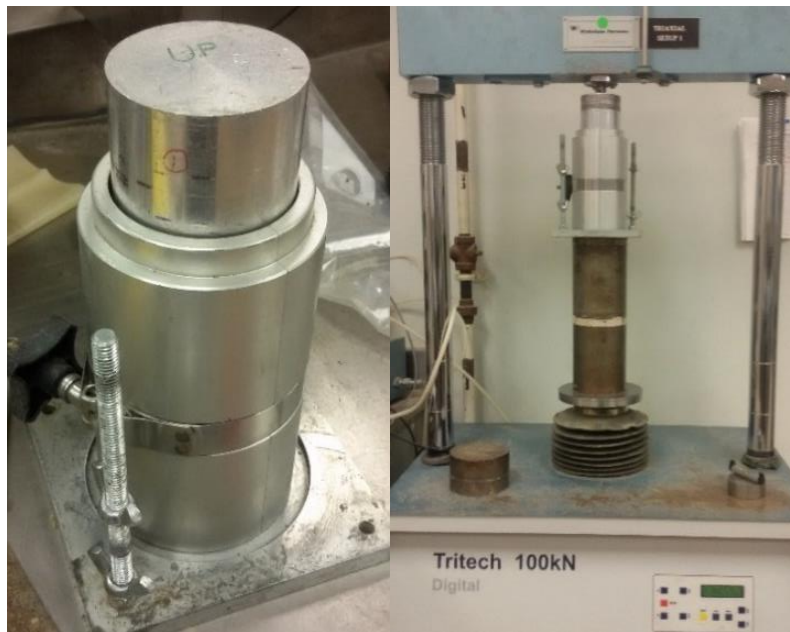
Figure 3-8 Compaction of UCS Sample
