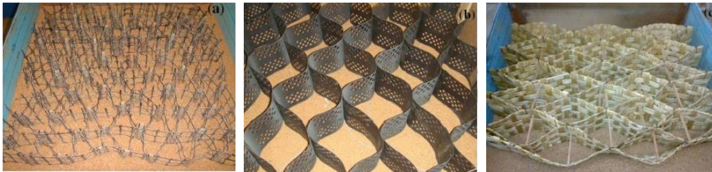
Figure 2.5 Three different confining systems used by Hegde and Sitharam for bearing capacity studies (a) geogrid cell (b) geocell (c) bamboo cell (Source: Hegde and Sitharam 2017)
