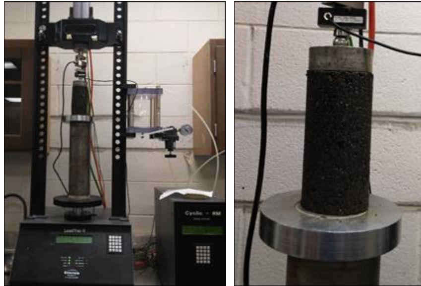
Figure 3.6 Equipment setup to perform UCS test on RAP sample
