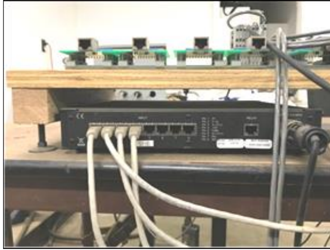
Figure 3.19 System 8000 StrainSmart data acquisition system (Saladhi 2017)
