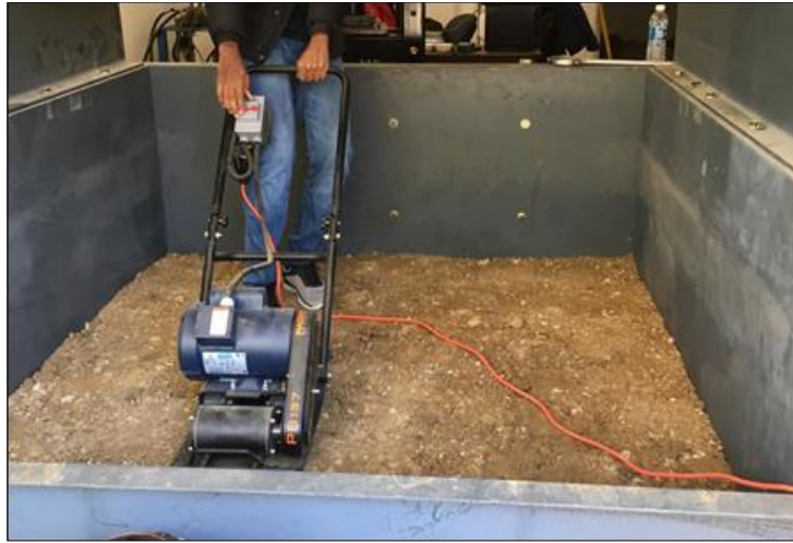
Figure 3.21 Compacting subgrade material using vibratory compactor
