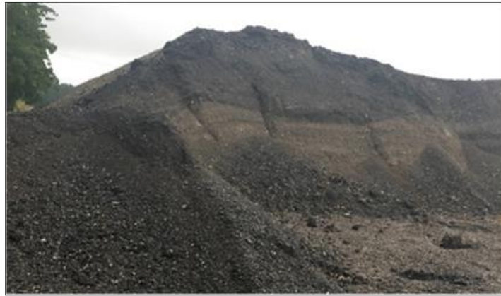
Figure 3.3 RAP stockpile at Grandview, Texas
