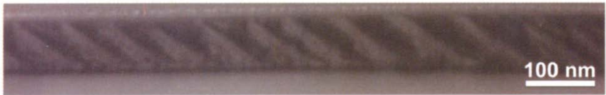
Figure 1. 2:(A) AFM image of BFO's MPB, consisting of alternating R-phase and Mc phase BFO. (B) Height variation of BFO along the MPB. (From [20])
