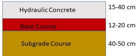
Typical Layers of a Rigid Pavement
