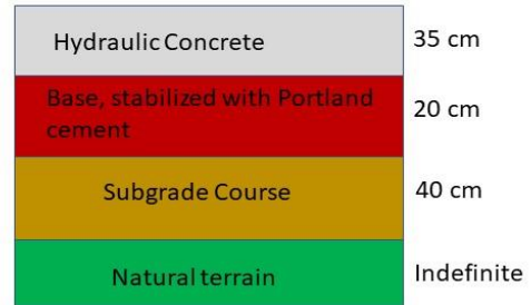
Rigid Pavement Layers For This Study
