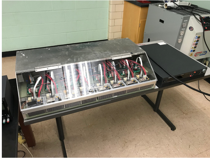
Figure 3.2: Completed and operational burn-in station (HV Supply shown to right)
