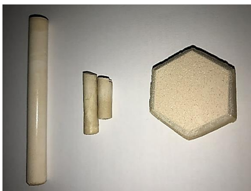
Figure 1.7 Metakaolin geopolymers synthesized in block form
