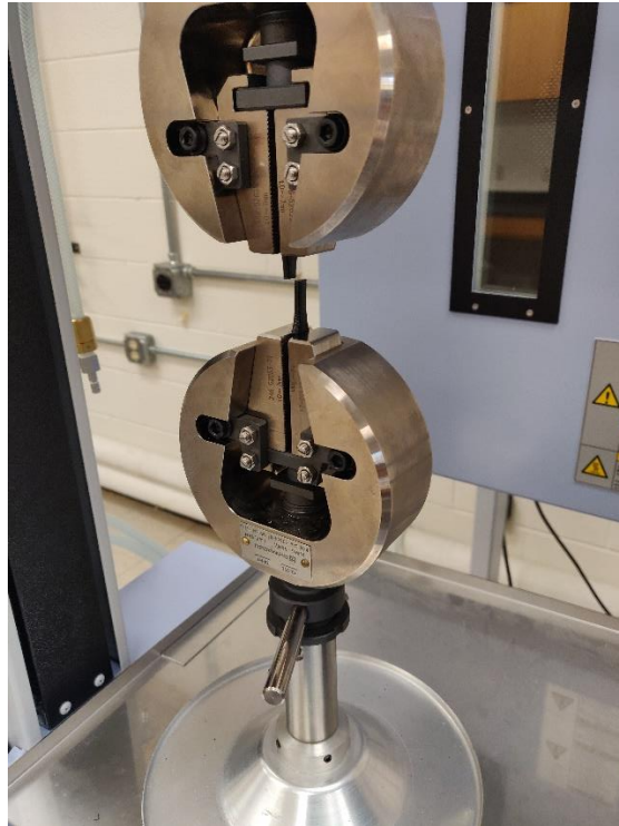
Figure 14: Tensile testing of dogbone specimens
