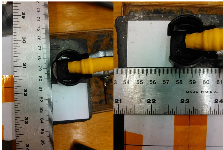
Figure 3-9 Left: initial image collected for the unblocked source in the x-direction; Right: Initial image collected for the unblocked source in the y- direction
