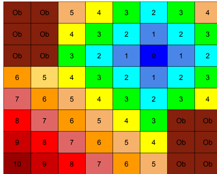
Figure A.1: Example result using the traditional wavefront expansion algorithm.
