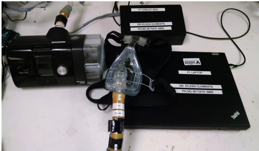
Figure 2.14 Leak Detector System Setup
