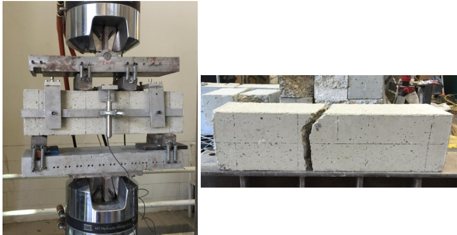
(a) (b) Figure 3-5. Flexural strength test on concrete beam: (a) test set up and (b) broken specimen (photo by Elmira Riahi)
