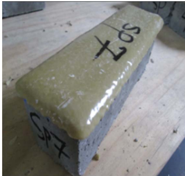
Figure 2-1 A typical coated beam specimen (image by Alimohammad Entezarmahdi)
