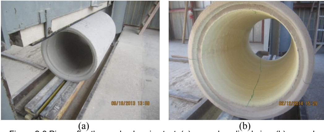
Figure 2-3 Pipes after three-edge bearing test: (a) example unlined pipe; (b) example lined pipe (image by Alimohammad Entezarmahdi)
