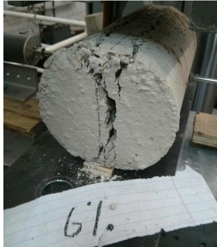
Figure 4-20 Failure of the cylindrical specimen at the end of the experimental splitting test
