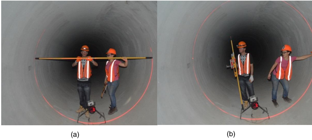
Figure 2-25 Video laser verification measurement (a) rod and (b) laser meter measurement for calculating the accuracy of the laser profiling method
