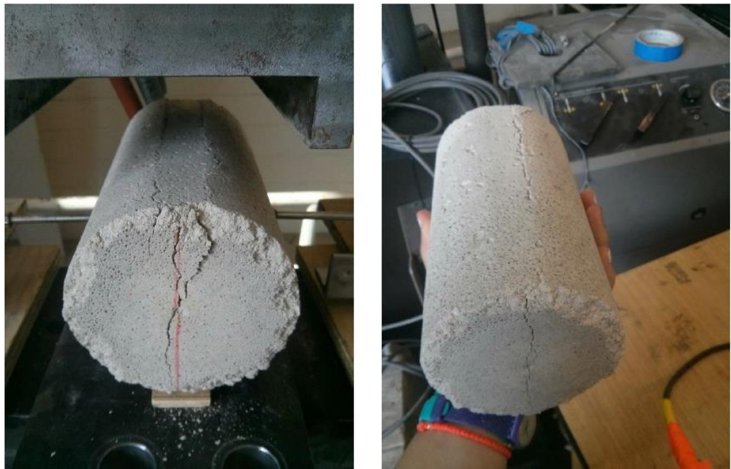
Figure 4-12 Failure pattern for the splitting tensile test
