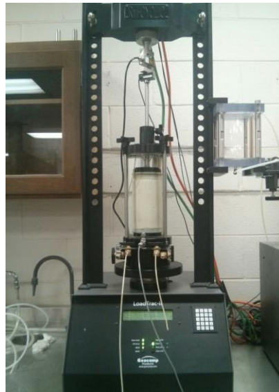
Figure 4-21 Confined triaxial test setup
