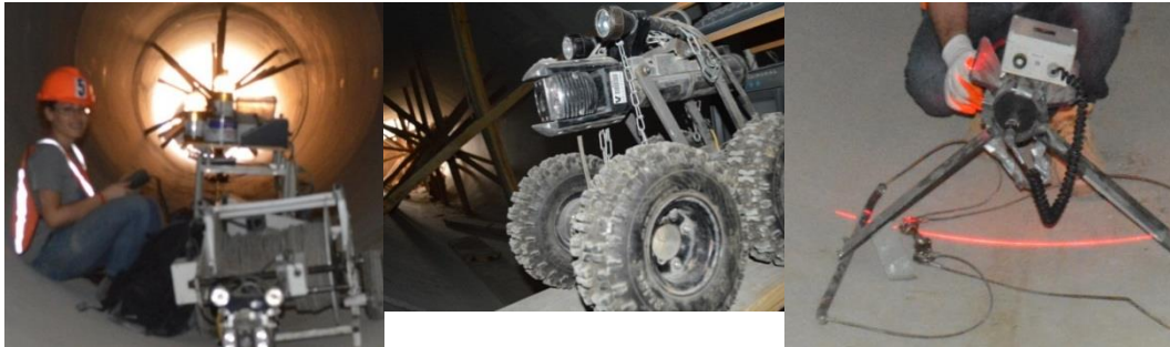
Figure 2-16 Video laser profiler equipment and connection for measurement
