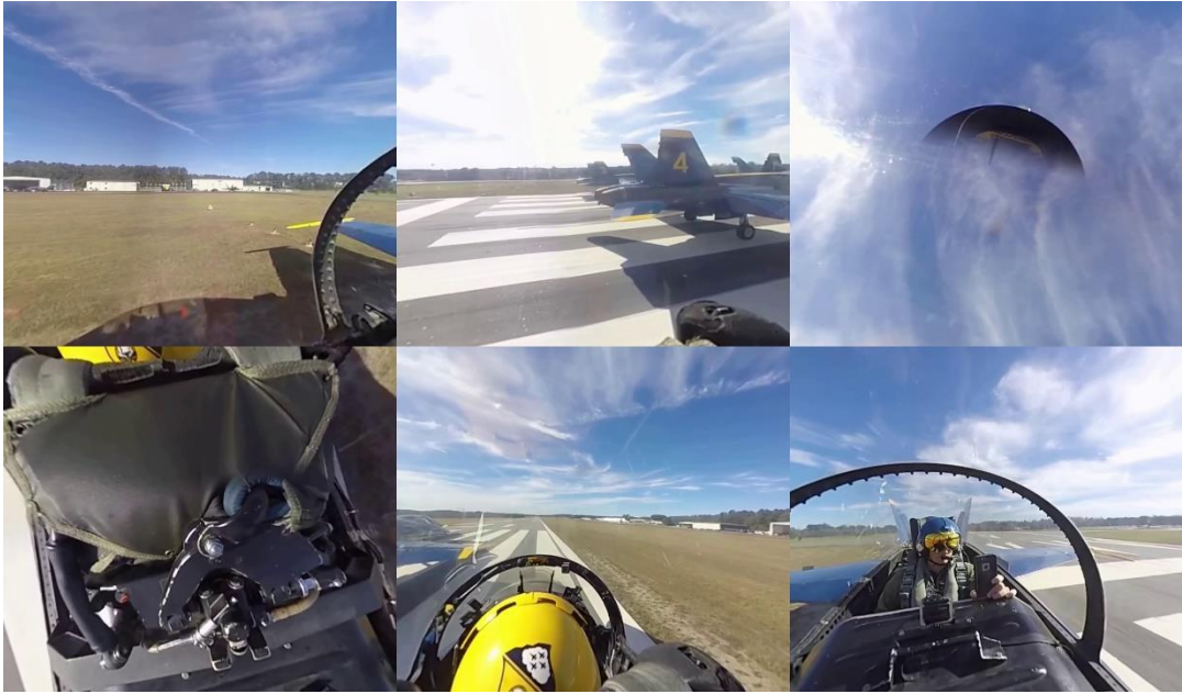
Figure 6.3b Frame packing for cube map projection
