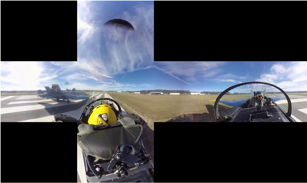
Figure 6.3a Example 360-degrees image that has been mapped into cubic
