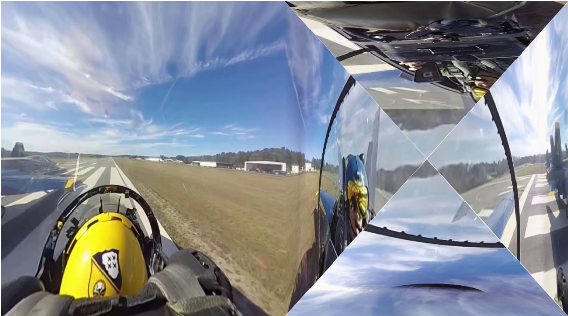
Figure 6.4b Rotation of side views and frame packing for Pyramid projection
