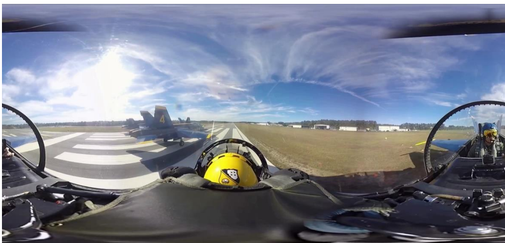
Figure 6.2 Example 360-degrees image that has been mapped into equirectangular
