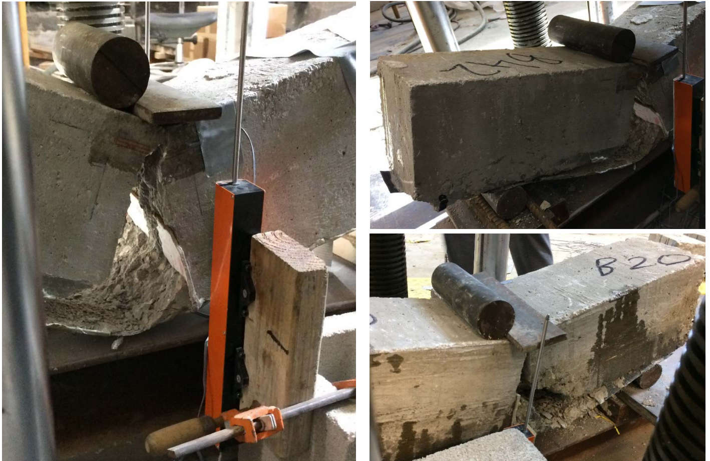
Figure 5- 23: Three points bending test failure
