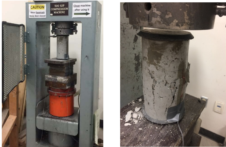
Figure 6- 6: ASTM cylinders compressive test setup
