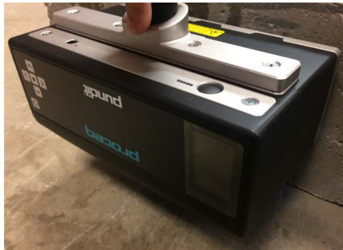
Figure 4- 34: Ultrasonic testing over the concrete surface
