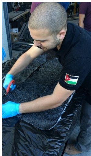
Figure 3-7: Cutting of the FRP
