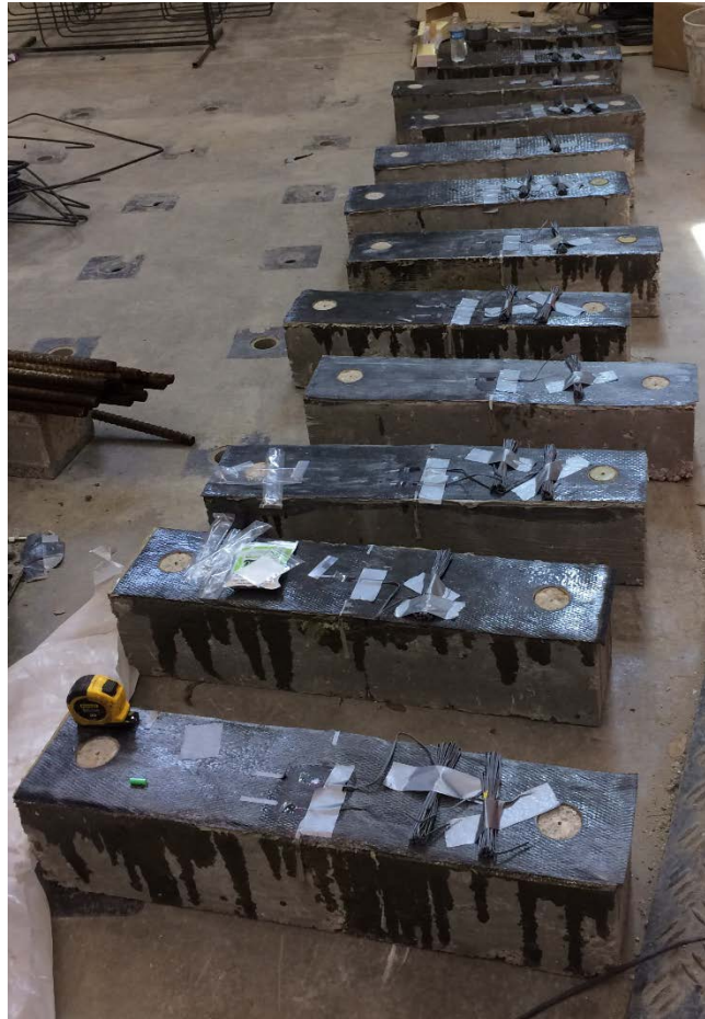
Figure 5- 20: Strain gages attached to the concrete beams
