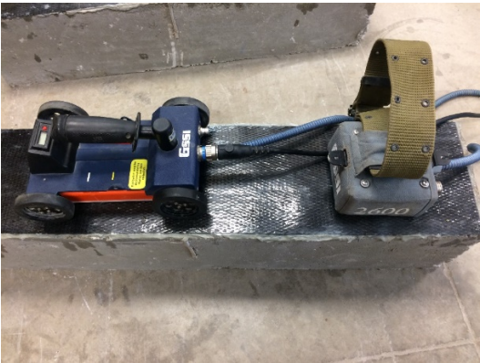
Figure 4- 49: 2600 MHz antenna connected to a mini-cart
