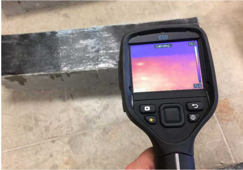
Figure 4- 26: Infrared camera used to capture pictures of the beam surface
