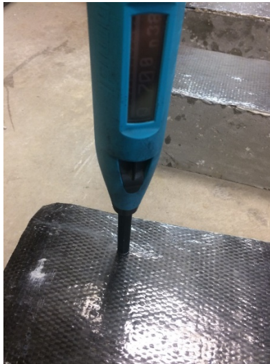
Figure 4- 4: Schmidt hammer testing at the FRP surface
