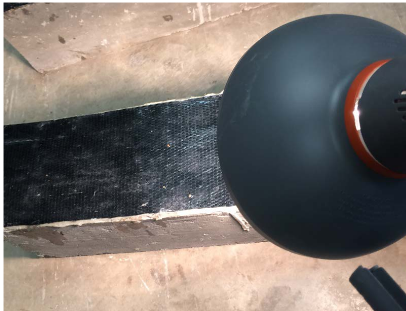
Figure 4- 25: Heating the beam using heat lamp
