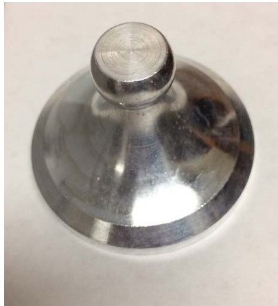
Figure 5- 5: Two inch diameter dolly
