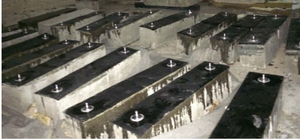
Figure 5- 7: Dollies attached to concrete surface
