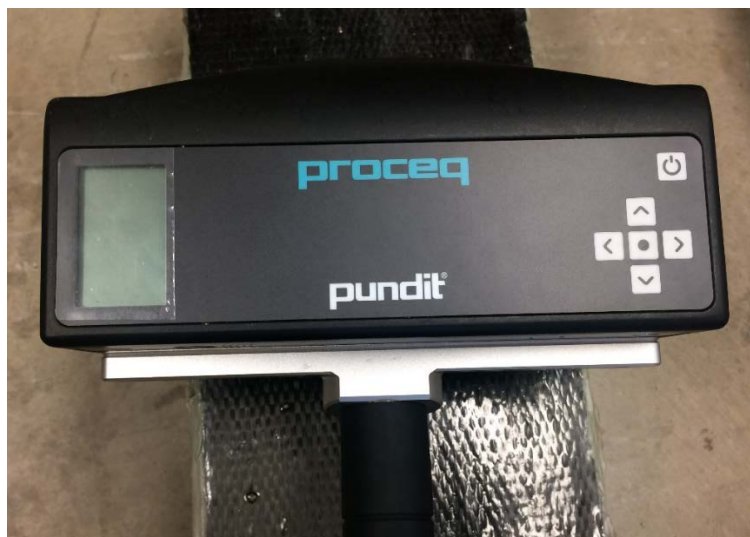
Figure 4- 33: Ultrasonic testing over the FRP surface
