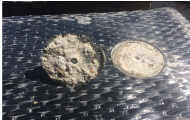
Figure 5- 9: Dolly pulled from beam surface
