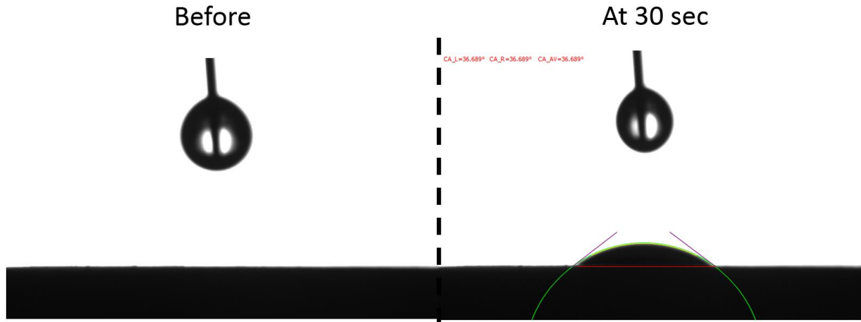
Figure 4-19 Before and after droplet of fluid on to sample surface, sample P1336-U 20%IPA
