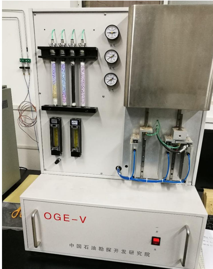
Figure 3-7 Instrument OGE-V for pyrolysis analysis
