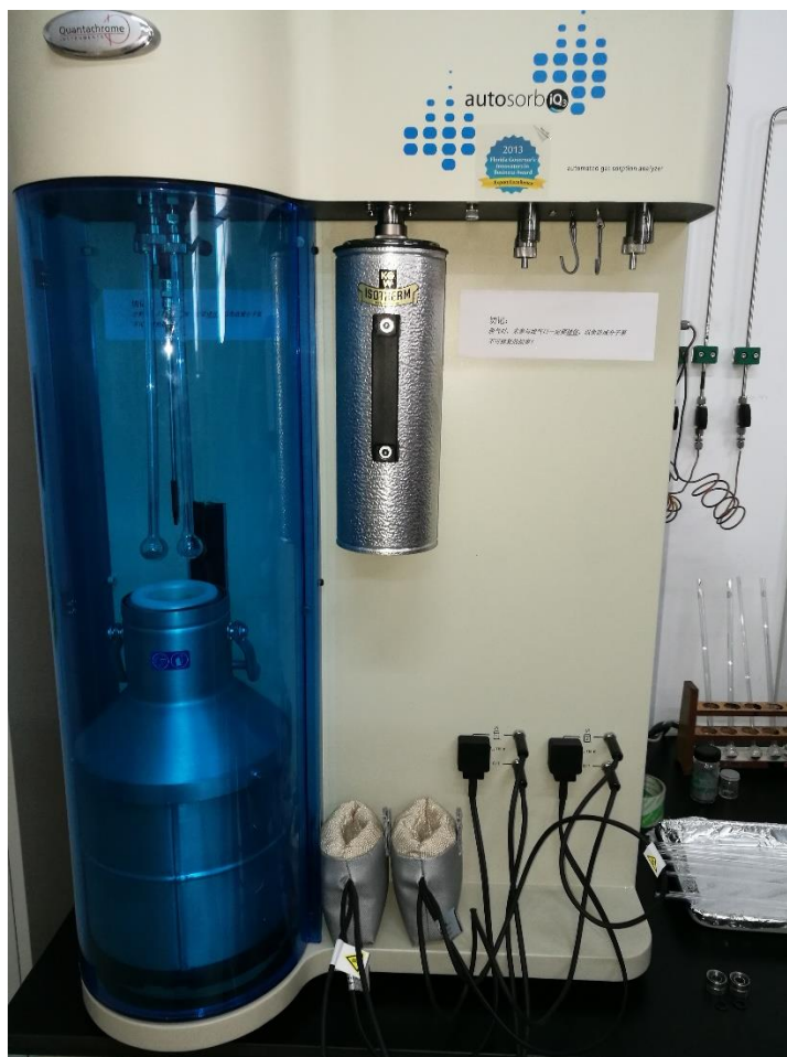
Figure 3-10 Autosorb iQ apparatus for low pressure gas physisorption
