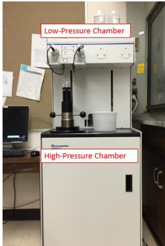
Figure 3-8 MICP apparatus of Micrometrics Autopore IV 9510
