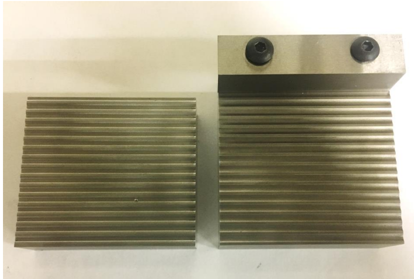
Figure 3-14 Thrust bearing bump foil tooling for radial bump foil arrangement
