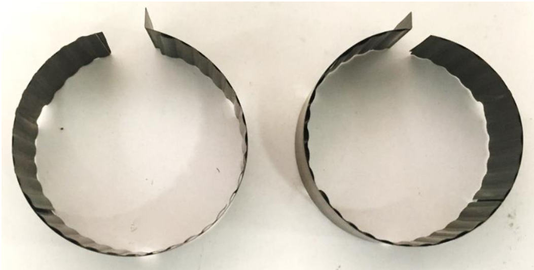
Figure 5-20 Split type bump foil stipes for case-1 single pad HAFB
