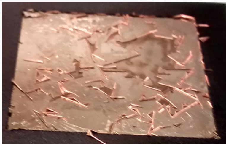
Figure S6-2 Spontaneous peeling and failure of nickel deposited from high chloride ( 600 \text{ g L}^{-1} ) plating bath.
