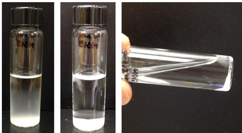
Figure 4-12. 1.9 \mu\text{m} C18 fully porous particles (Titan) suspended in ethanol. The particles are allowed to settle after sonication (preferably overnight) and the bed is examined by tilting the vial. Note how the bed slides down the base of the vial. A loose bed (shown above) is an indicator of a bad slurry. Indeed, EtOH produced very poor columns regardless of the slurry concentration (80,000 N/m plates vs. 210,000 N/m plates using a dispersive suspension).
