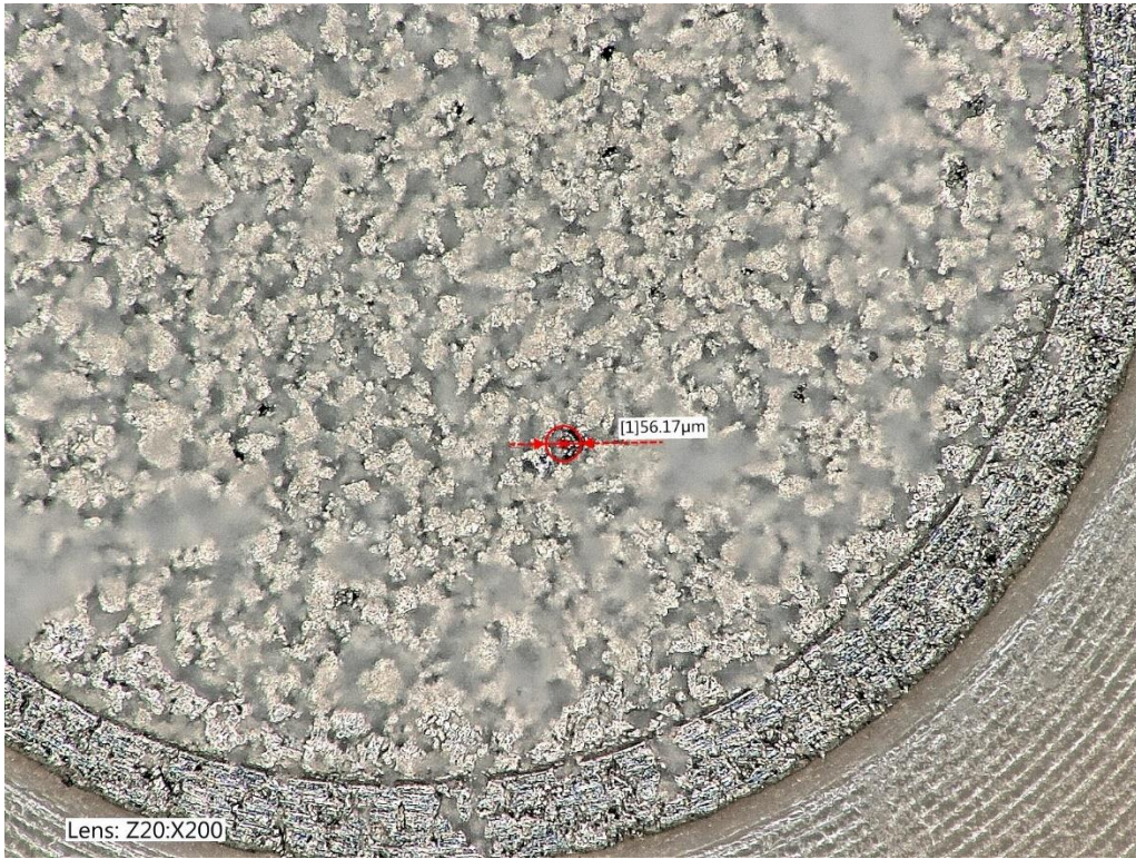
Figure 4-4. A high-resolution image of the PEEK based frit from Figure 4-3(B) after it had been exposed to 10,000 psi during a packing. A 56.17 \mu\text{m} diameter hole appeared on the surface when the damaged frit was removed from the column. The manufacturer lists the specification of the frit to be above 10,000 psi. Image taken using Keyence VHX digital microscope using Z20 lens with 200x magnification.
