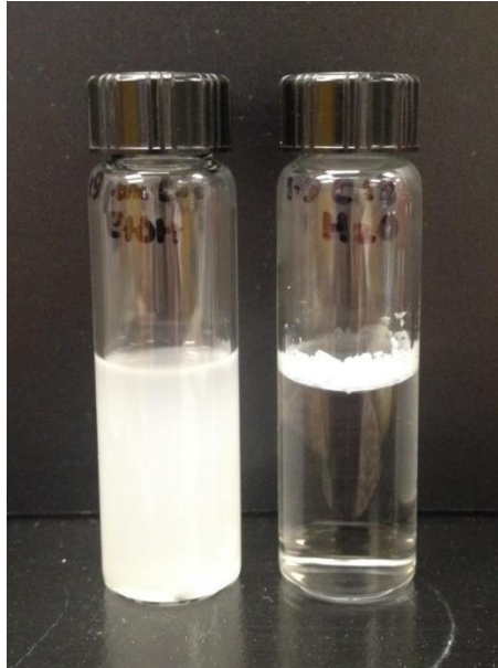
Figure 4-7. 1.9 \mu\text{m} C18 phase dispersed in ethanol (left) and water (right). This is an example of creaming. Although ethanol is able to wet the phase, it is highly agglomerating; therefore, not a suitable suspension medium.
