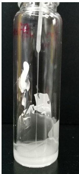
Figure 4-13. A thick suspension of C18 1.9 \mu\text{m} FPP silica showing a filament formed when picked up with a pipette.
