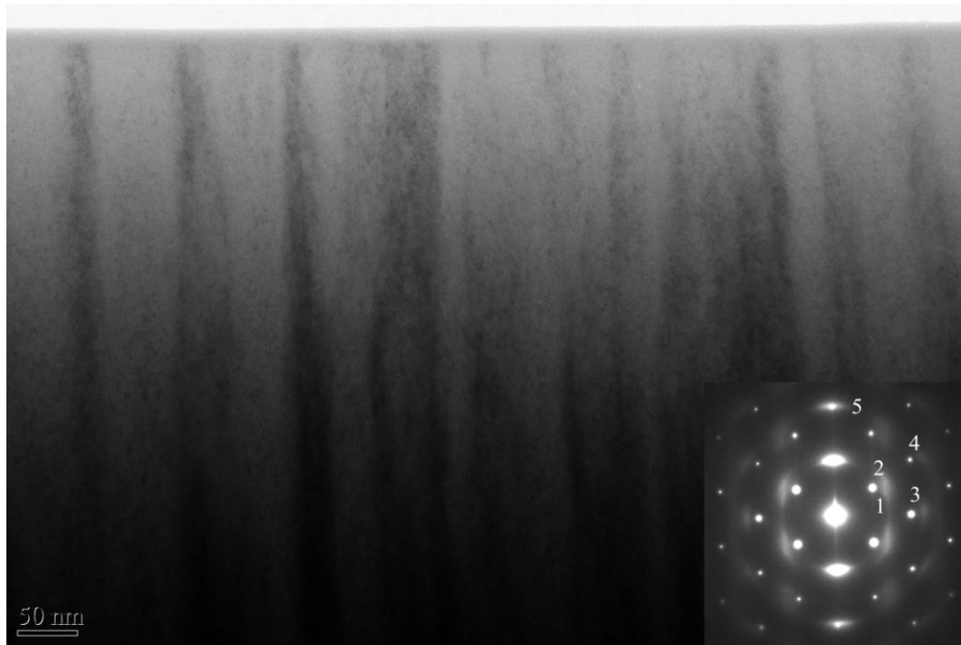
Fig. 4.2.5. Cross-section bright field TEM image of the Zr_{61}B_{27}C_6N_3 coating with inserted SAED taking from the interface of coating and substrate.
