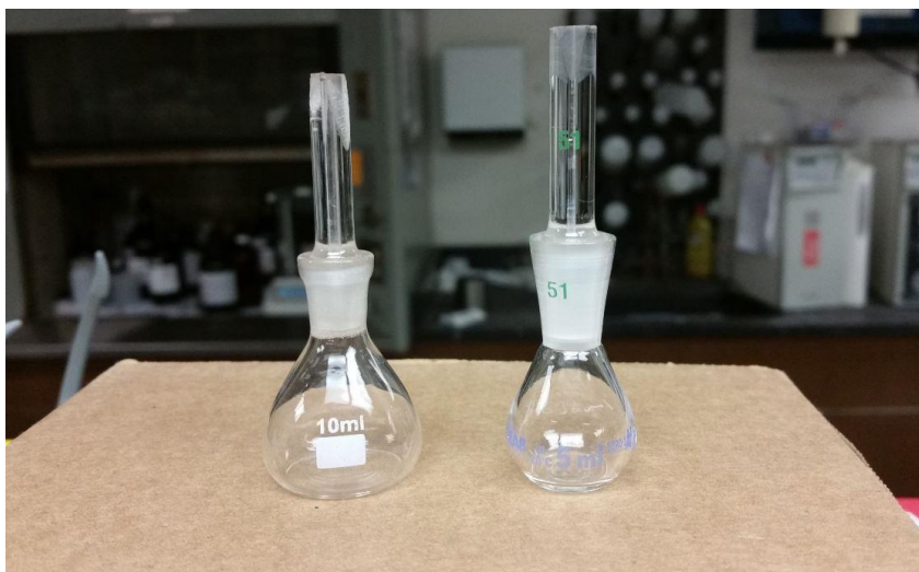
Figure 3-6: Stopped bottles for pycnometry experiment
