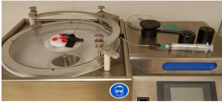
Figure 3.11 - Spin coating chamber with attached solvent injection nozzle.
