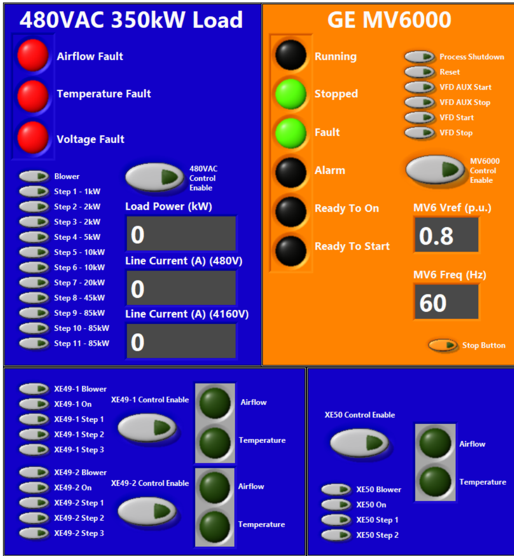
Figure 4.22: The VI used for controlling the Mosebach load units and the MV6. This VI is split into four quadrants – one for the 480 VAC load bank, one for the two 6 kVDC load banks, one for the 12 kVDC load banks, and one for the MV6 unit.
