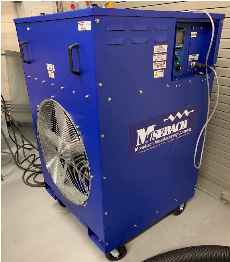
Figure 4.14: Photograph of the Mosebach 350 kVA - 480 VAC resistive electronic load installed in the laboratory.
