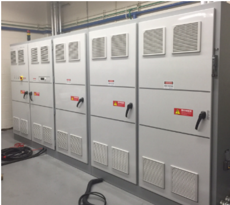
Figure 2.24: Photograph of UTA's 1200V/700A/500kW Chroma 17030 battery cycler.
