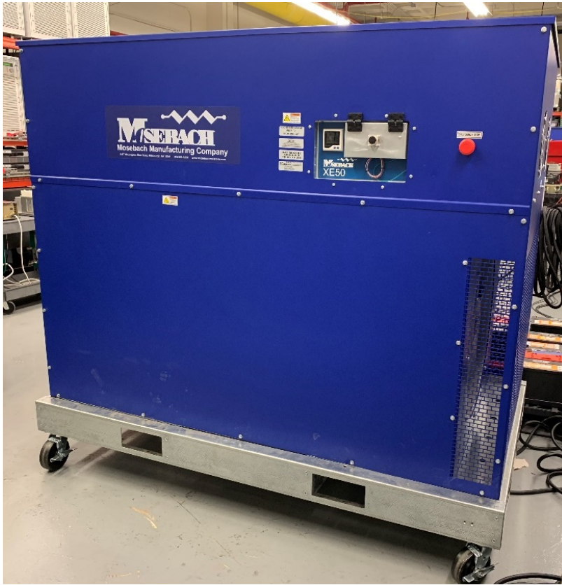
Figure 4.9: Photograph of the 12 kVDC – 100 kW resistive load.
