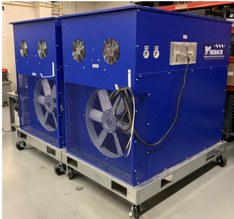
Figure 4.18: Photograph of the two 6 kVDC – 150 kW resistive loads.
