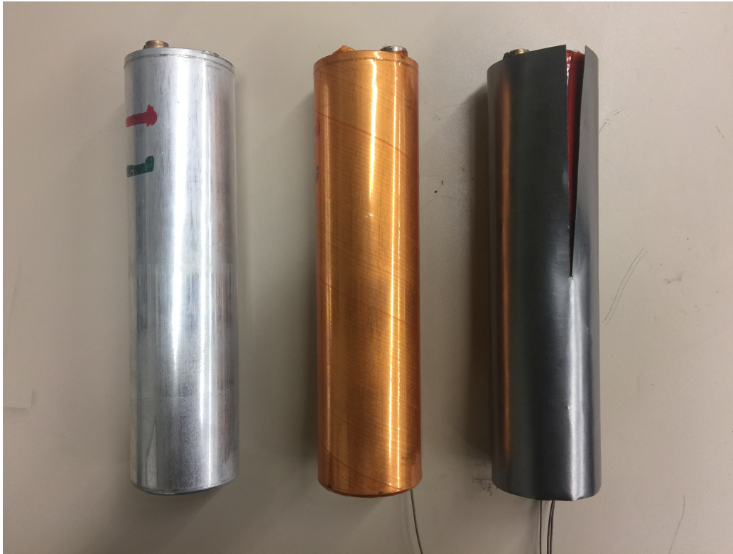
Figure 2.14: Photographs showing the bare cell (left), the cell wrapped in mylar heatshrink (middle), and the mylar wrapped cell covered in graphite thermal interface material (right).
