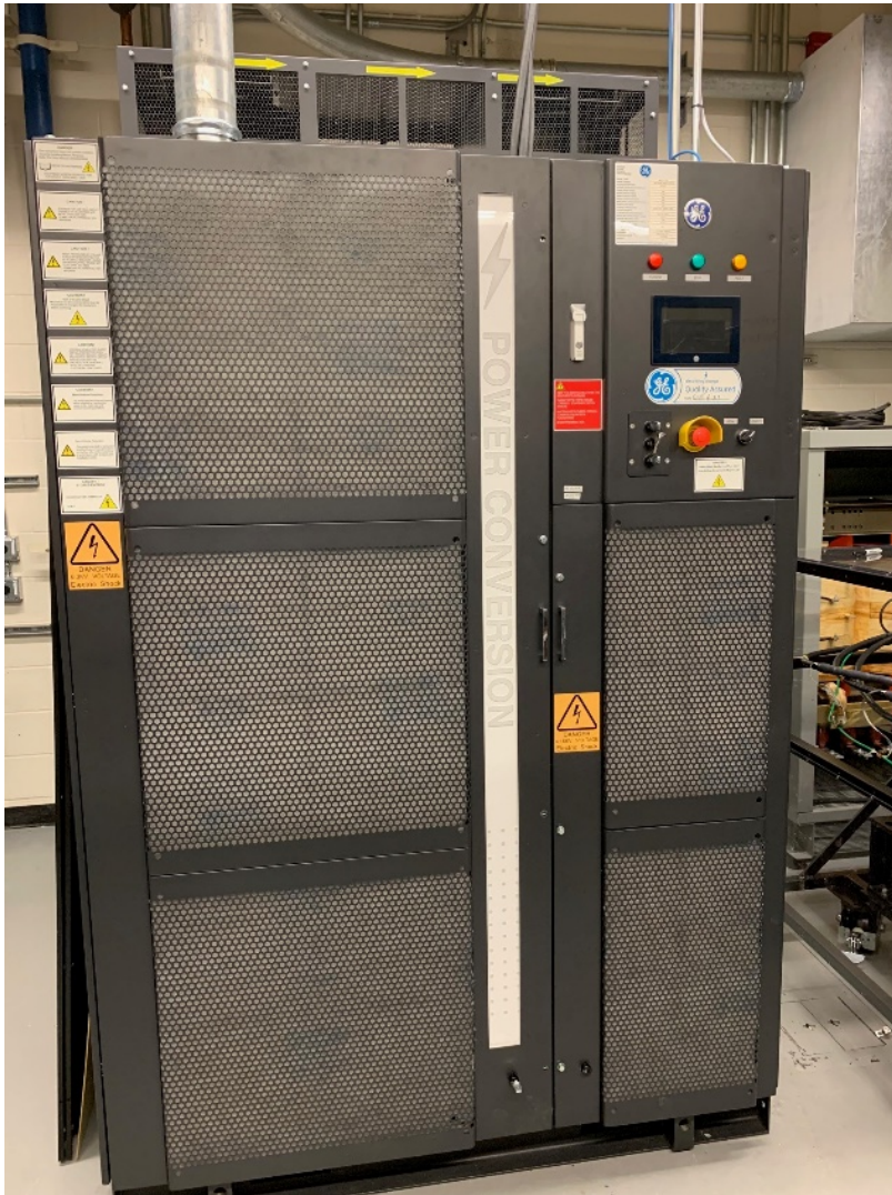
Figure 4.10: Photograph of the GE MV6000 power electronic drive.
