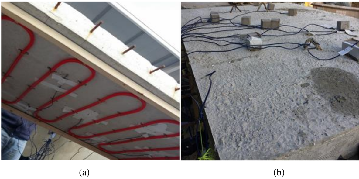
Figure 5- 3 (a) Pipes Enclosed within Wooden Framework, (b) Complete thermocouple Set-up
