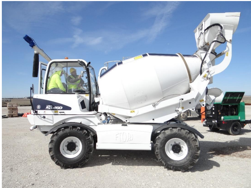
Figure 5- 3 High-shear mixer used for the UHP-FRC mixing.
