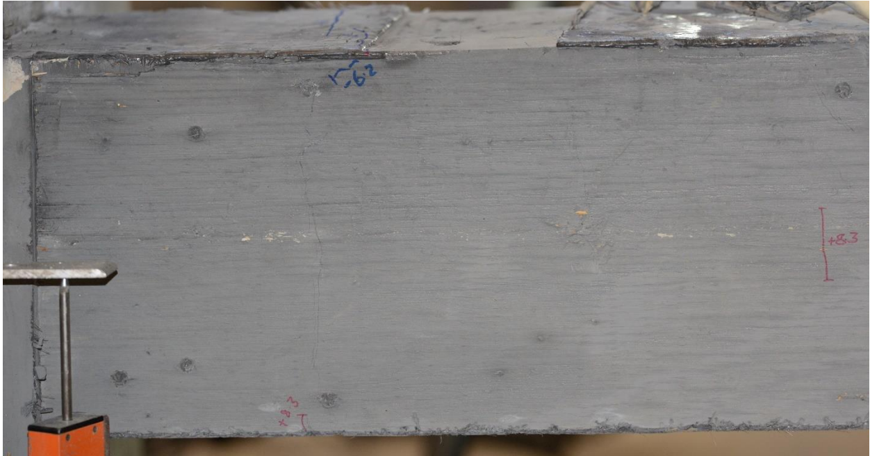
Figure 9- 72 UHP-FRC #4 at 0.75% drift
