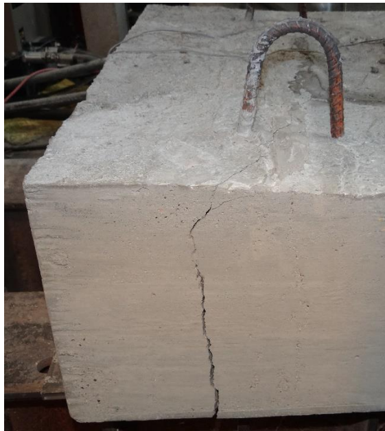
Figure 4- 21 Throughout cracks observed near the slab ends propagating from the corner of the inner slabs.
