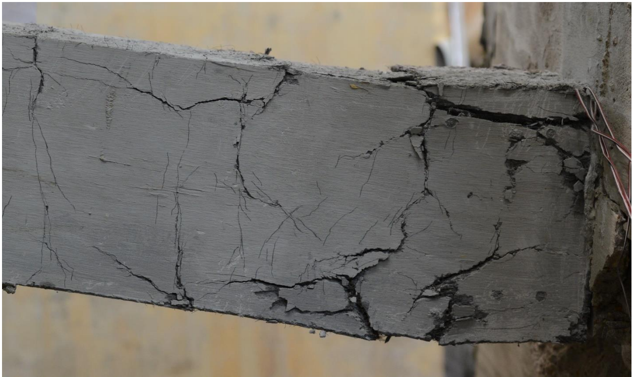
Figure 9- 40 UHP-FRC #2 at 15.0% drift
