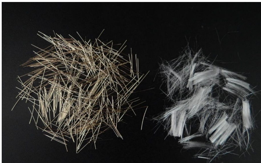
Figure 3- 1 Micro steel fiber (left) and ultra-high molecular weight polyethylene fiber (right).
