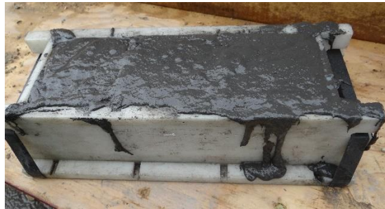
Figure 5- 7 Collection of UHP-FRC samples for compressive testing
