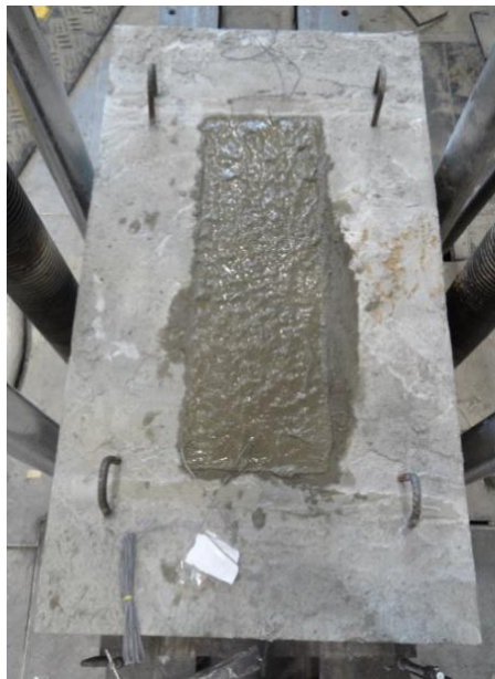
Figure 3- 23 Cast in place PC punch test specimen.
