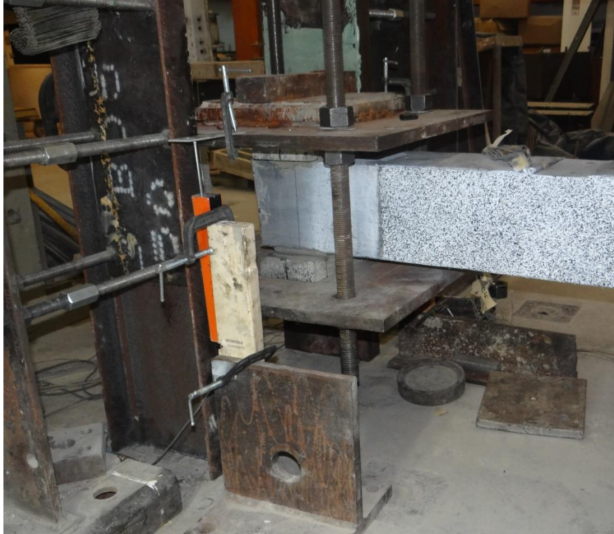
Figure 8- 33 Figure showing the loading head setup of the cantilever specimen
