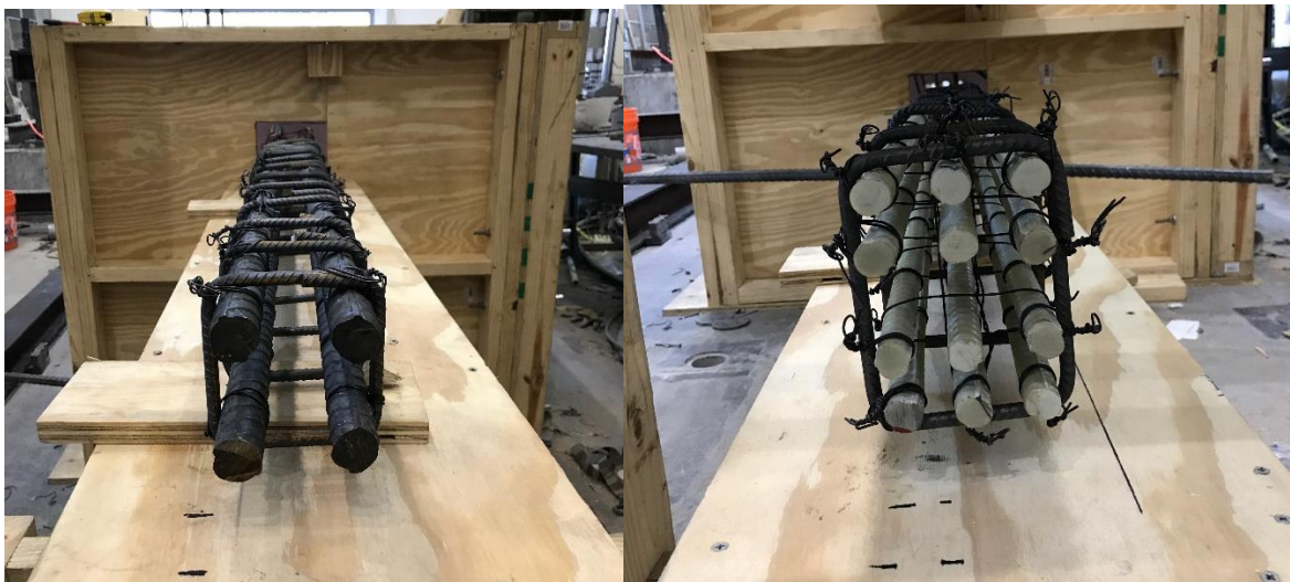
Figure 8- 23 Reinforcement for specimens UHP-FRC #1 (left) and UHP-FRC #2 (right)
