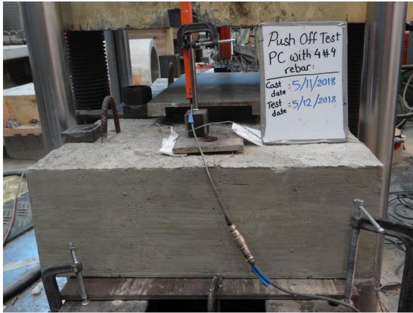
Figure 3- 30 Test setup for the punch test.
