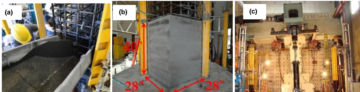
Figure 7- 12 (a) UHP-FRC casting at UT Arlington CELB, (b) completed UHP-FRC at the plastic hinging zone of the specimen, and (c) experimental testing at MAST laboratory at the University of Minnesota
