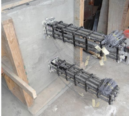
Figure 8- 26 The hardened concrete of the support block shown with the specimen (UHP-FRC #3 and UHP-FRC #4 specimen BFRP reinforcements)
