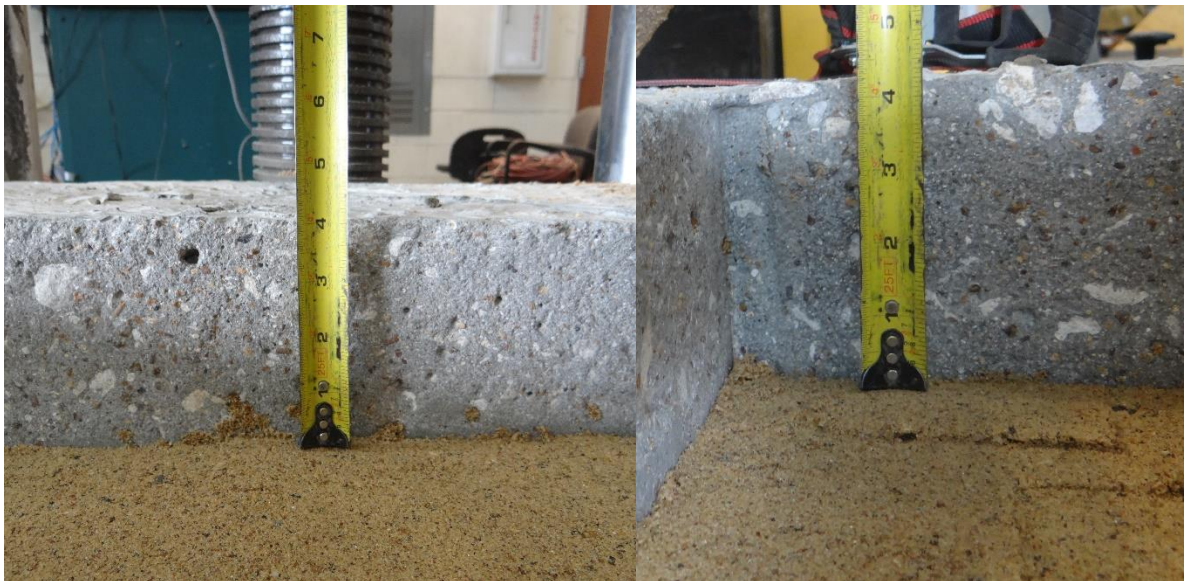
Figure 3- 26 The 4-inch casting surface level obtained after placement and compaction of sand in the hollow portion.
