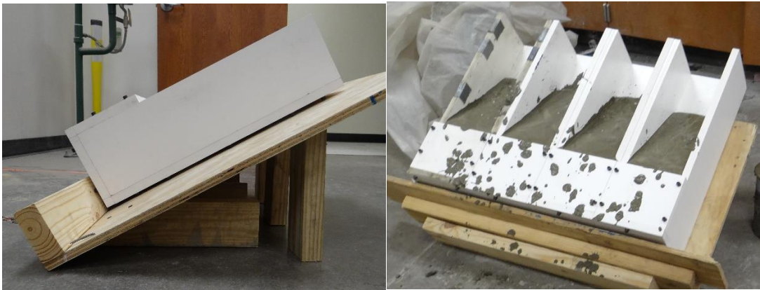
Figure 3- 3 Mold placement and casting for bottom half of slant shear specimen.
