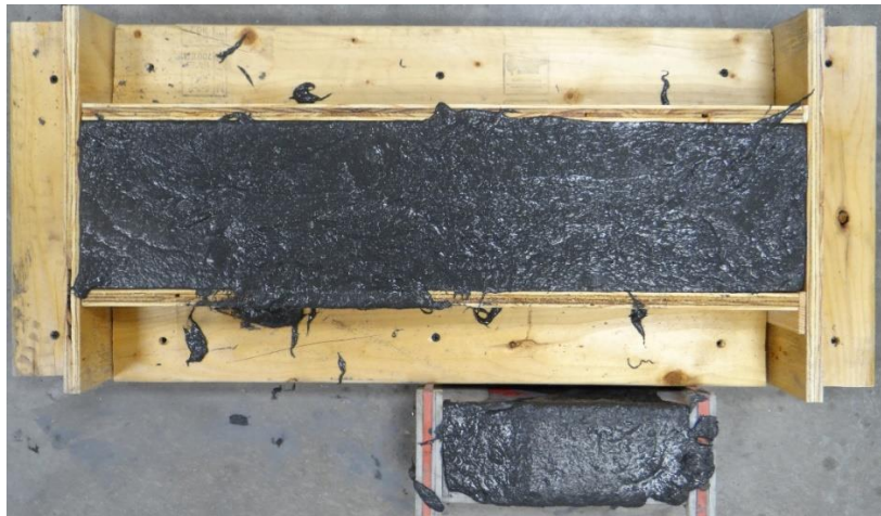
Figure 3- 24 Formwork and casting of the UHP-FRC precast panel.
