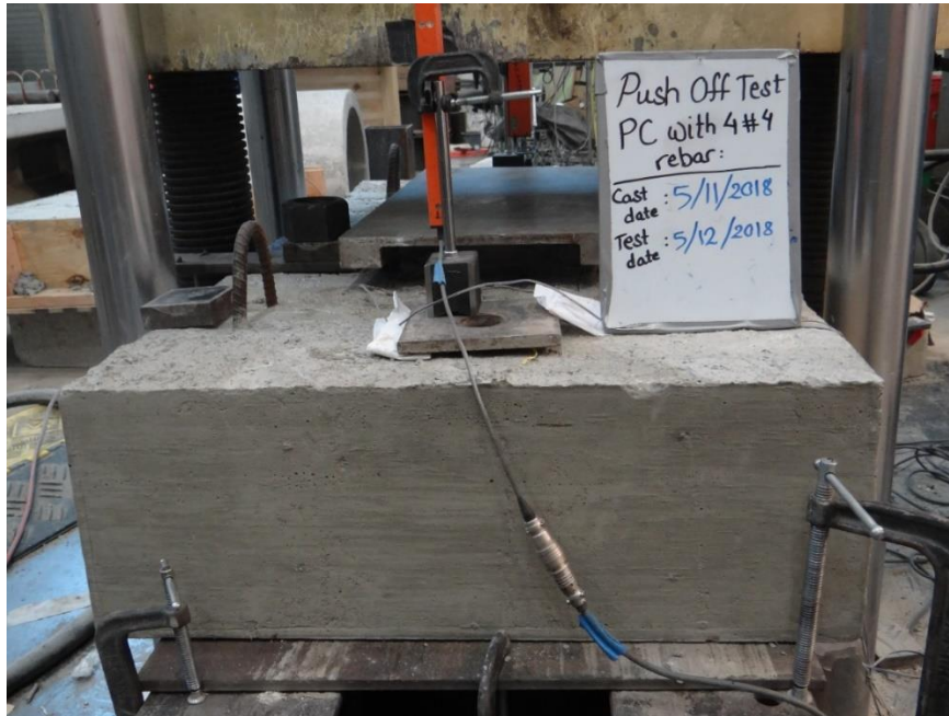
Figure 4- 17 Punch test setup for PC specimen with dowel bars.
