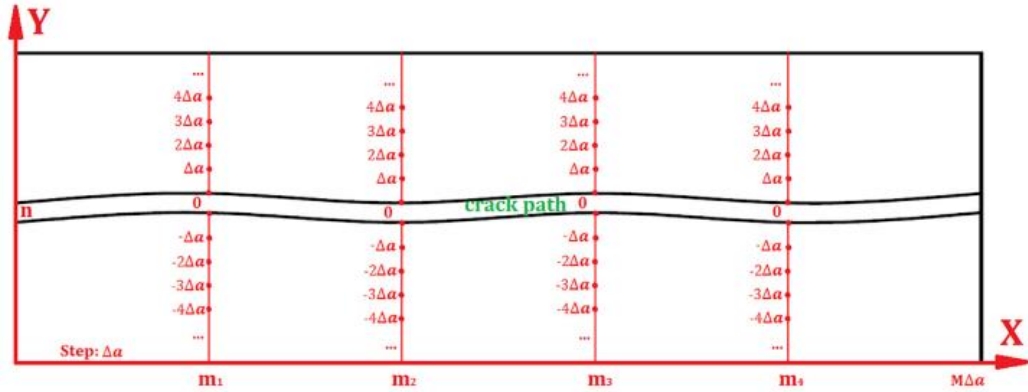
Figure 4-21 Schematic representation of the post mortem crack path analysis proposed by Rui et al (76).
